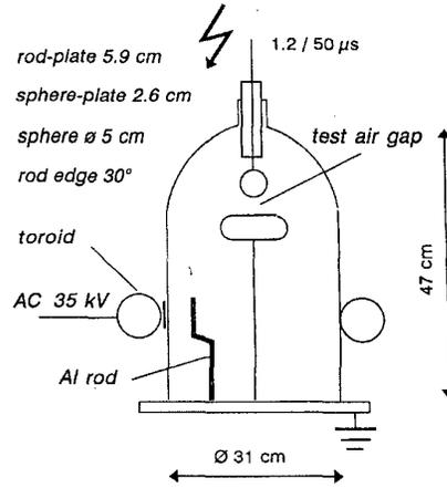
Figure 3. Model test setup.
