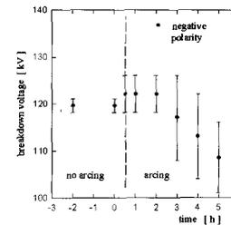
Figure 8. Electrical strength changes at the rod-plane gap, negative polarity.
