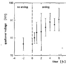
Figure 4. Increase of arrester sparkover voltage during internal arcing test.
