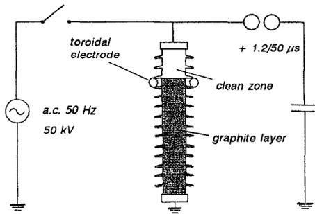
Figure 2. The arrester under internal arcing test.
