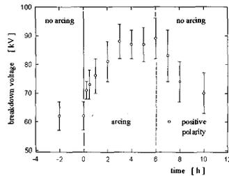
Figure 5. Electrical strength changes at the sphere-plane gap, positive polarity.
