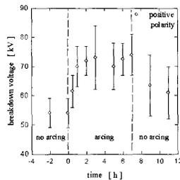
Figure 6. Electrical strength changes at the rod-plane gap, positive polarity.
