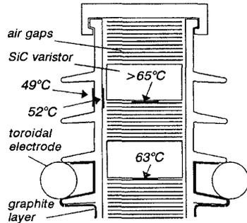
Figure 1. The arrester's longitudinal section.
