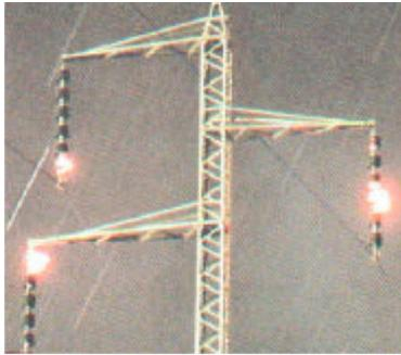
Fig. 6. Discharges on 110-kV line insulators in Israel [17].
