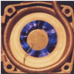
Fig. 2. Intensive partial discharges inside a surge arrester.
