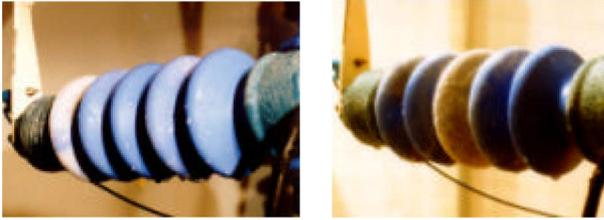
Fig. 4. Dry band changes on a porcelain insulator with silicone rubber coating during the accelerating aging test according to IEC standard 61109 [9].
