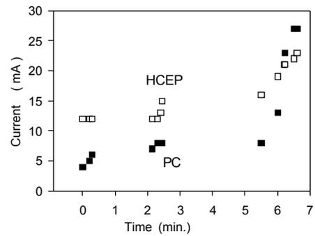
Fig. 5: Currents on PC insulators and on hydrophobic cycloaliphatic epoxy insulators (HCEP) recorded on 1.05.2006
