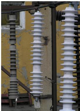
Fig. 4: Medium voltage insulator chains tested at Glogow station. Hydrophobic epoxy insulator (on the left) and polymer concrete insulators (in the centre and on the left).
