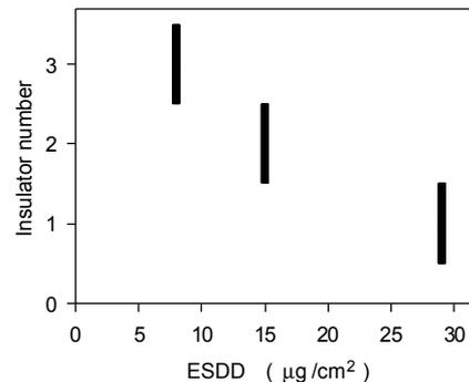
Fig. 3: ESDD on the damaged string consisted of three insulators.. The top insulator has the number 3.
