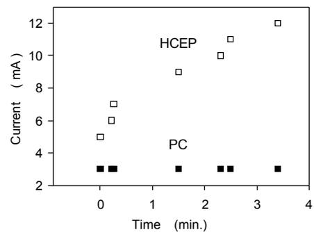
Fig. 6: Currents on PC insulators and on hydrophobic cycloaliphatic epoxy insulators (HCEP) recorded on 16.05.2006
