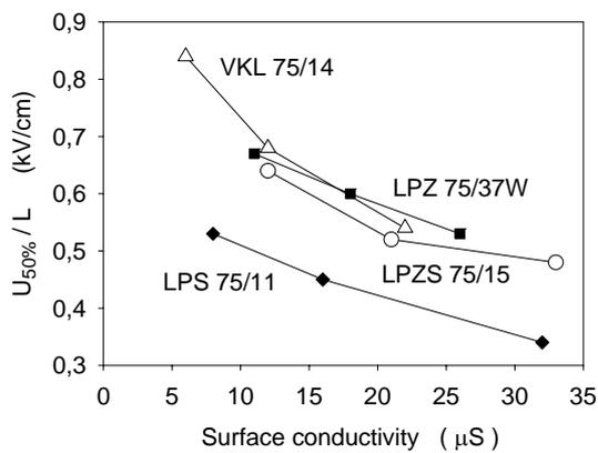
**Fig. 8** Pollution characteristics measured according to flow on method
