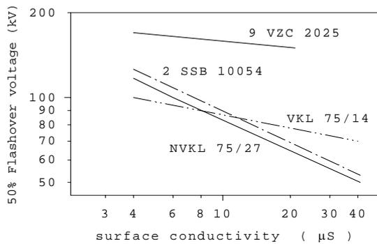
**Fig. 5** Pollution characteristics of 4 selected insulators obtained in steam fog [9]
