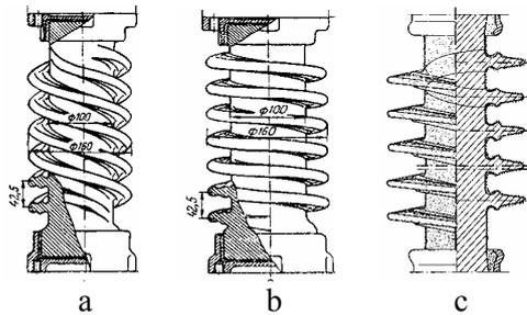
**Fig. 3** The profiles of spiral insulators: a; b – soviet insulators of series CT-35 [6]; c – polish insulator LPZS 75/11
