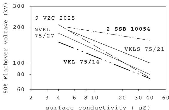
**Fig. 6** Pollution characteristics of insulators obtained according to flow on method with methylcellulose layer [9]
