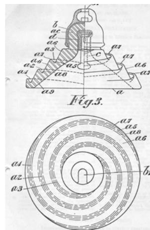
Fig. 2 The cap and pin insulator with a spiral rain-pipe on the shed [12]
