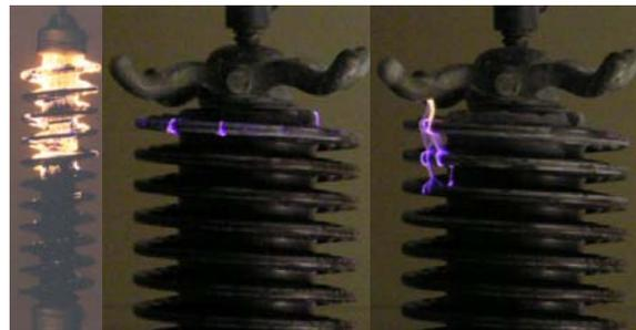
**Fig. 9** Discharges on insulators with spiral sheds during flow on test. a – insulator LPS 75/11; b, c – insulator SSB 10054
