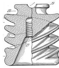
Fig. 1 The Stroup insulator with spiral shaped sheds [11]
