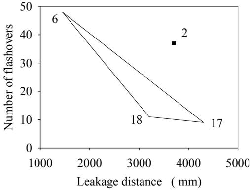
**Fig. 7** Flashover number as a function of leakage distance of support insulators. Point 2 - Insulator with spiral sheds [7]
