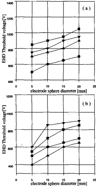
Figure 3: Electro-convection threshold voltage in fresh oil versus the electrode sphere diameter, for different coating materials when both electrodes are coated (a) and when only the sphere is coated (b): (●) uncoated electrodes, (▲) coating with Teflon, (■) coating with Silicon oxide, and (▼) coating with Silicon nitride; the electrode sphere being positive.
