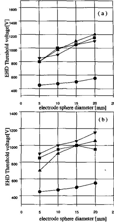
Figure 4: Electro-convection threshold voltage in aged oil versus the electrode sphere diameter, for different coating materials when both electrodes are coated (a) and when only the sphere is coated (b): (●) uncoated electrodes, (▲) coating with Teflon, (■) coating with Silicon oxide, and (▼) coating with Silicon nitride; the electrode sphere being positive.
