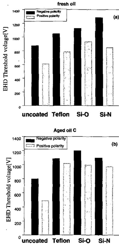
Figure 5: Electro-convection threshold voltage for electrodes uncoated and coated with Teflon, Silicon oxide and Silicon nitride, for both polarities of the electrode sphere: (a) fresh oil, (b) aged oil.
