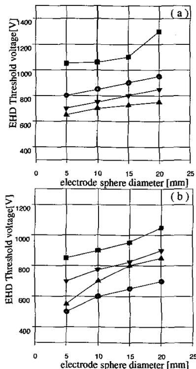
Figure 2: Electro-convection threshold voltage in fresh oil versus the electrode sphere diameter, for different configurations of electrodes coating with Silicon oxide for a negative sphere (a) and a positive sphere (b): (●) uncoated electrodes, (▲) sphere coated with Silicon oxide, (■) both electrodes coated with Silicon oxide, and (▼) electrode plane coated with Silicon oxide.
