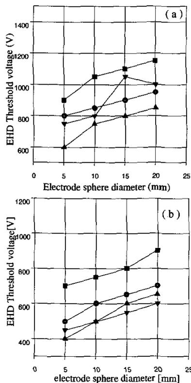
Figure 1: Electro-convection threshold voltage in fresh oil versus the electrode sphere diameter, for different configurations of electrodes coating with Teflon for a negative sphere (a) and a positive sphere (b): (●) uncoated electrodes, (▲) sphere coated with Teflon, (■) both electrodes coated with Teflon, and (▼) electrode plane coated with Teflon.
