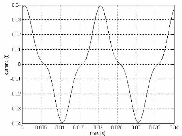
Fig. 4a. The varistor current (supply voltage  $U$  is distorted by 3rd odd harmonic)
