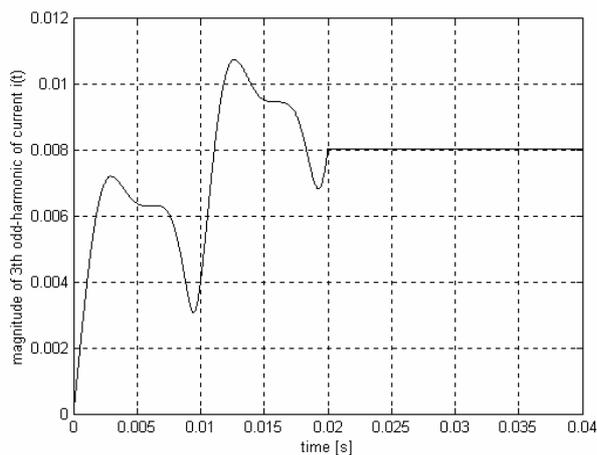
Fig. 4b. The magnitude of 3rd odd-harmonic of the varistor current (supply voltage  $U$  is distorted by 3rd odd harmonic)
