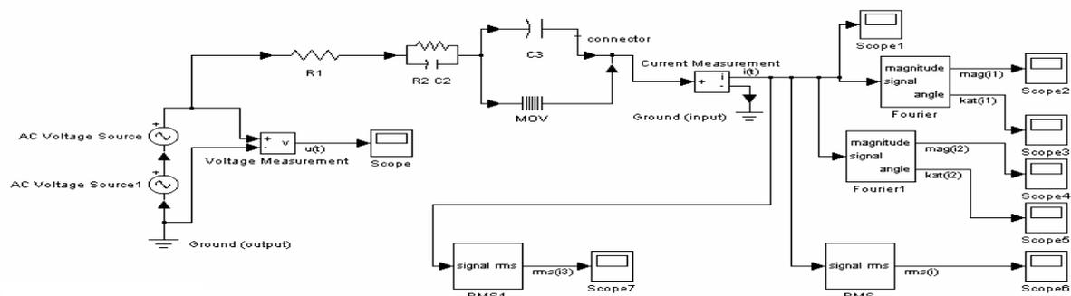
Fig. 1. The implementation of varistor model in Matlab program.
