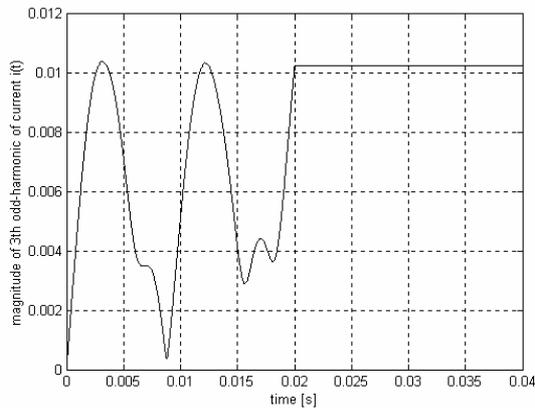
Fig. 2b. The magnitude of 3rd odd-harmonic of the varistor current for  $U > U_c$
