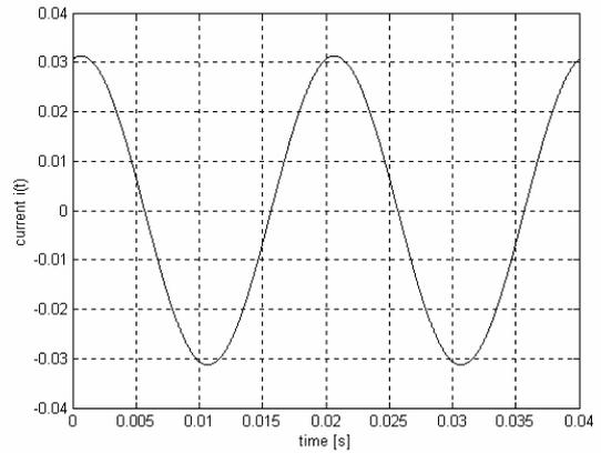
Fig. 3a. The varistor current for  $U < U_c$
