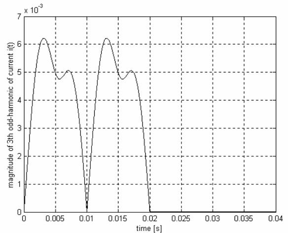
Fig. 3b. The magnitude of 3rd odd-harmonic of the varistor current for  $U < U_c$
