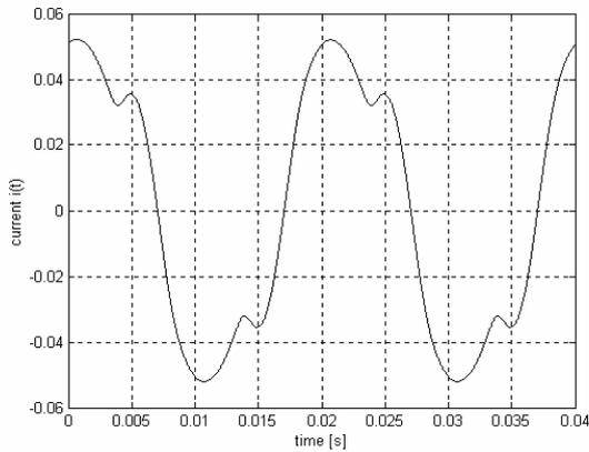
Fig. 2a. The varistor current for  $U > U_c$
