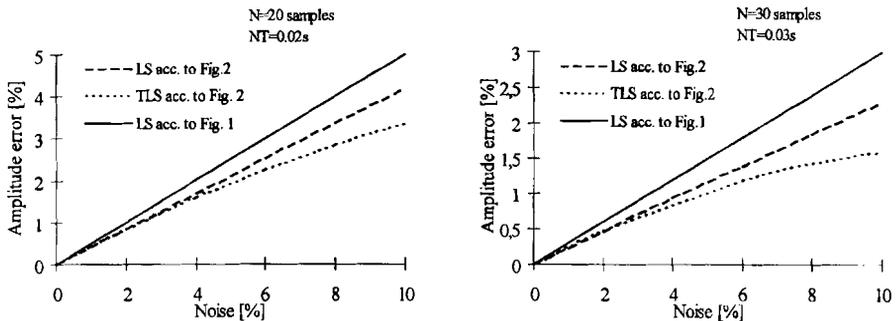
**Figure 3.** Errors of the amplitude estimation when using the networks acc. to Figure 1 and acc. to Figure 2
