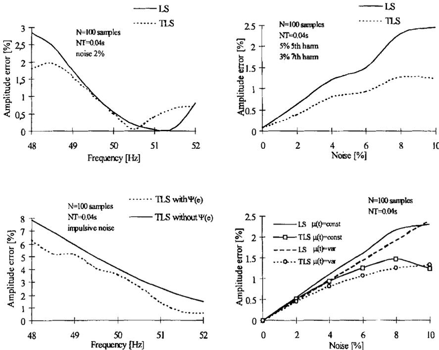
**Figure 4.** Errors of the amplitude estimation of the new method (Figure 2)
