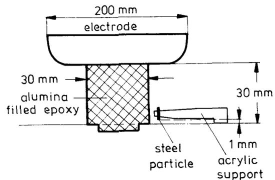
Figure 1. Geometry of the test gap.
