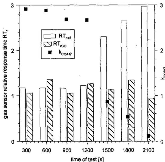
Figure 5. Variation of  $k_{CO/H_2}$  and  $RT_r$  for "hot spot" simulation.
