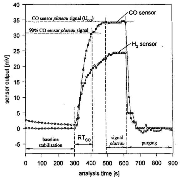
Figure 2. Gas sensor output waves recorded during analysis run.
