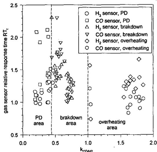
Figure 4. Identification of transformer fault type.
