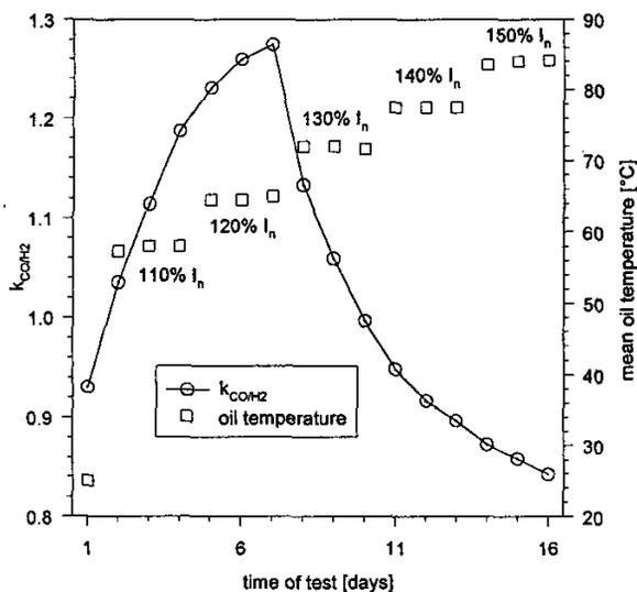
Figure 6. Rate of  $k_{CO/H_2}$  change during transformer overload test.
