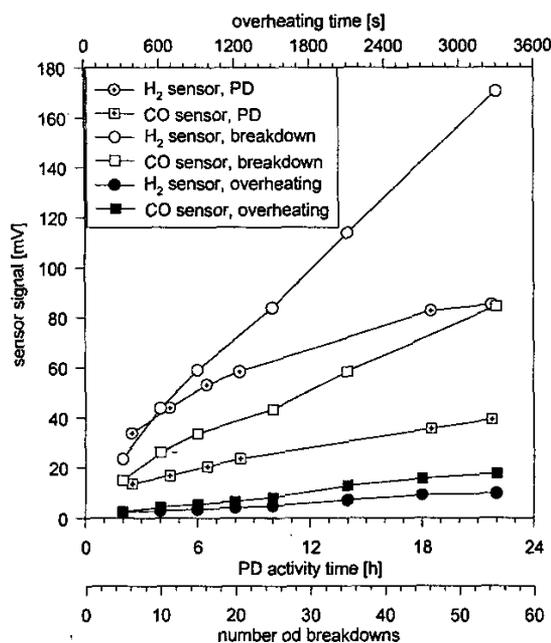
Figure 3. Rate of gas sensor output rise for simulated fault types.
