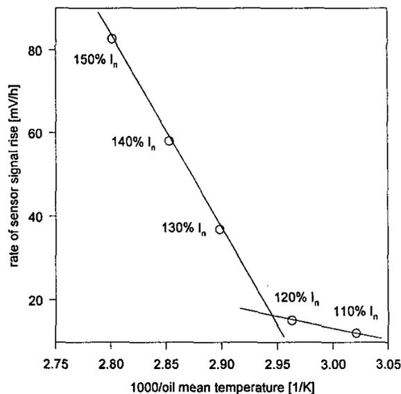
Figure 7. *Arrhenius* plot for overload test data.
