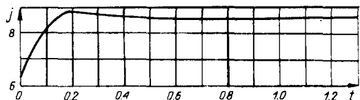
Fig. 1. Time-varying wave form of current density j(t) in the system of normalized variables
