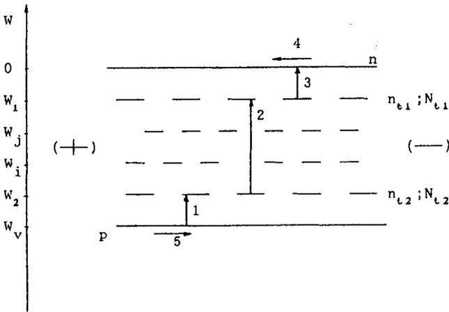
**Figure 1.** The energy diagram and allowed electron transitions caused by incident phonons and photons, where  $W$  is the total energy of the electron,  $W_v$  is the valence level, and (+) and (−) denote the anode and cathode, respectively: 1,  $\nu_p N_{t2}$  with the hole activation energy denoted by  $(W_2 - W_v)$ ; 2,  $C_{21} n_{t2}$ ; 3,  $\nu_n n_{t1}$  with the electron activation energy denoted by  $-W_1$ ; 4,  $\mu_n nE$ ; 5,  $\mu_p pE$ .
