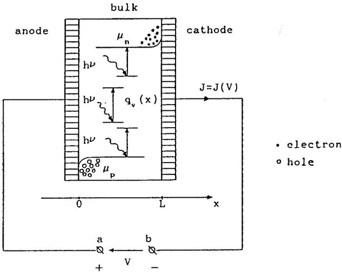
**Figure 2.** The planar capacitor system and the boundary and internal processes. Here,  $h\nu$  denotes the total energy of a phonon and a photon;  $q_v(x)$  is the space charge distribution and  $J$  is the total current density; a and b denote the voltage (or current) terminals.
