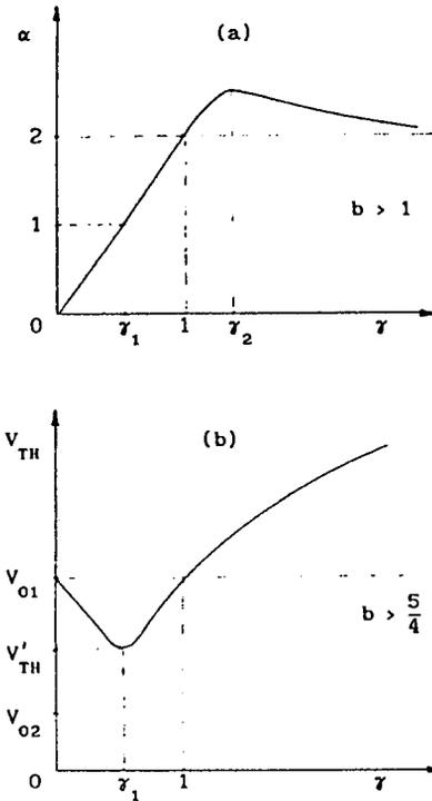
Figure 4. The importance of the parameters  $\alpha$  and  $V_{TH}$  for the switching effect: (a) the shape of the function  $\alpha = \alpha(\gamma)$ ; (b) the shape of the function  $V_{TH} = V_{TH}(\gamma)$ .
