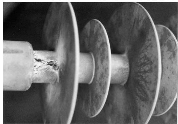
Fig. 6. Composite insulator after long duration ageing in rain chamber.
