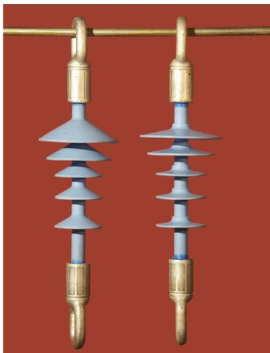
Fig. 1: ‘Inverted Christmas tree’ design of composite insulators: with shed inclination of 30° (left) and with shed inclination of 10° (right).
