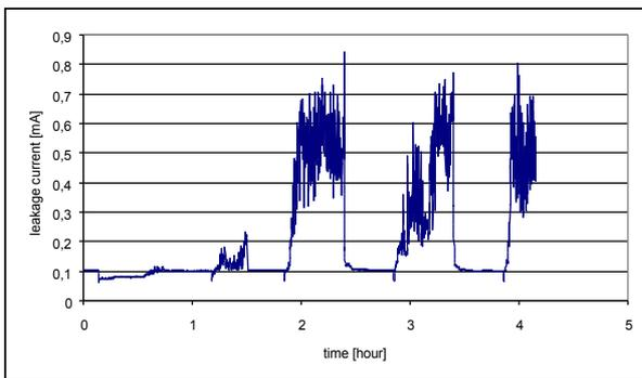
Fig. 4. Leakage current registered on 7th day of insulator 6c10 ageing in rain chamber. Test voltage 24 kV.
