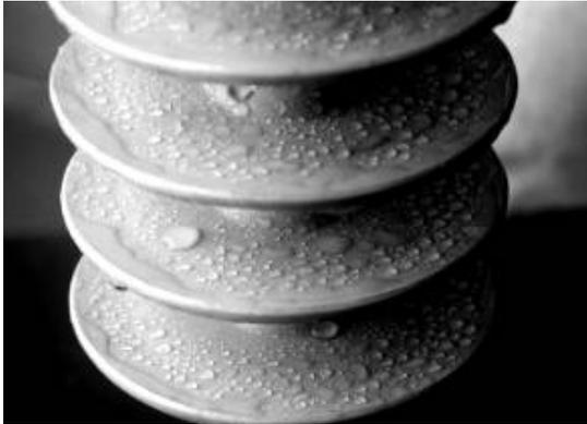
Fig. 3. Undersides of insulator 6c10 on sixth day of ageing in rain chamber.
