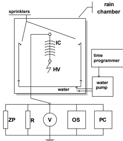
Fig. 2: Schematic of rain chamber system: IC – silicone rubber insulator, PC – personal computer, V – digital voltmeter, OS – digital scope, R – measuring resistor, ZP – overvoltage protection.
