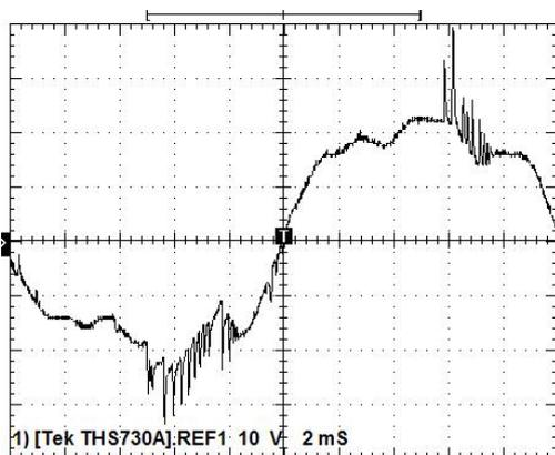
Fig. 5. Instantaneous traces of leakage current for insulator 6c10 on 7th day of ageing. Test voltage 24 kV.
