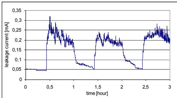
Fig. 7. Leakage current registered on 65th day of ageing insulator 6c30 in rain chamber. Test voltage 40 kV.
