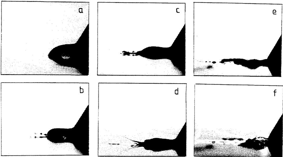
Fig.4. The instability of the water drop located on the hydrophobic surface before the flashover: drop volume  $20 \mu\text{l}$ , AC non-uniform electric field.
