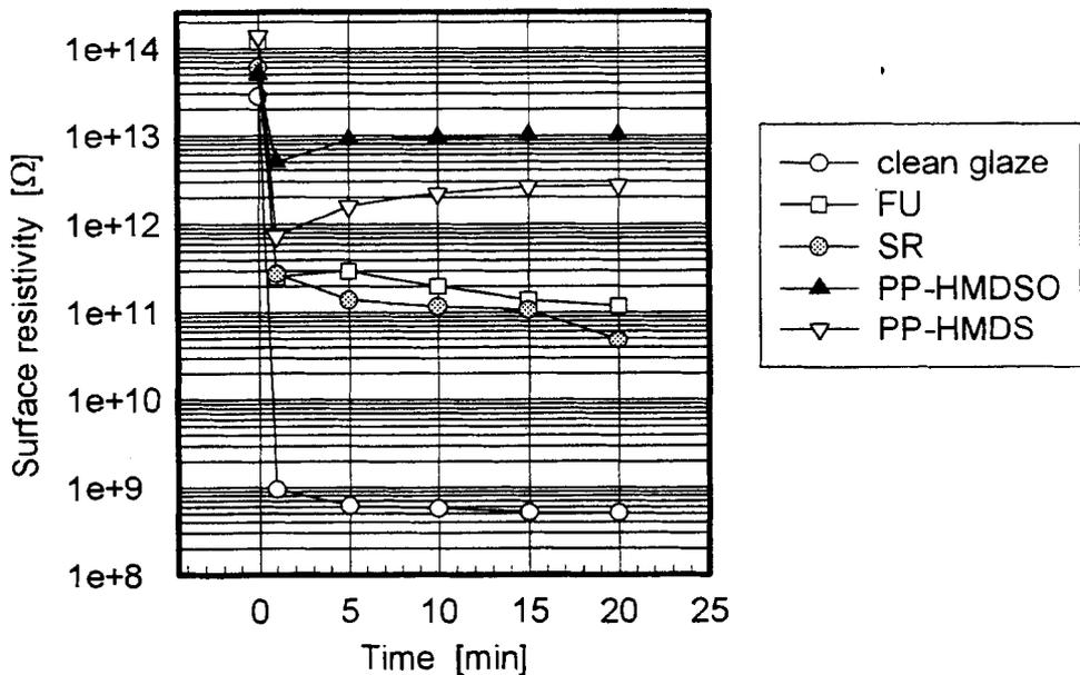
Fig. 2. Surface resistivity versus the wetting time in the small fog chamber: SR - silicon rubber coating, FU - fluorourethan coating, PP - plasma modified samples.
