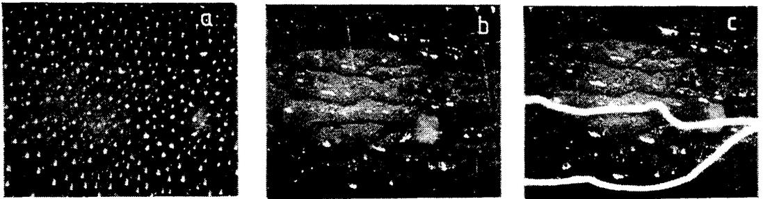
Fig. 5. The formation of the water channels and the flashover under AC voltage.
