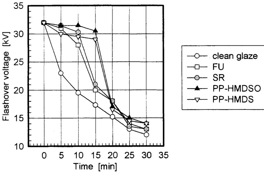
Fig.3. AC flashover voltage versus of the wetting time in the fog chamber.
