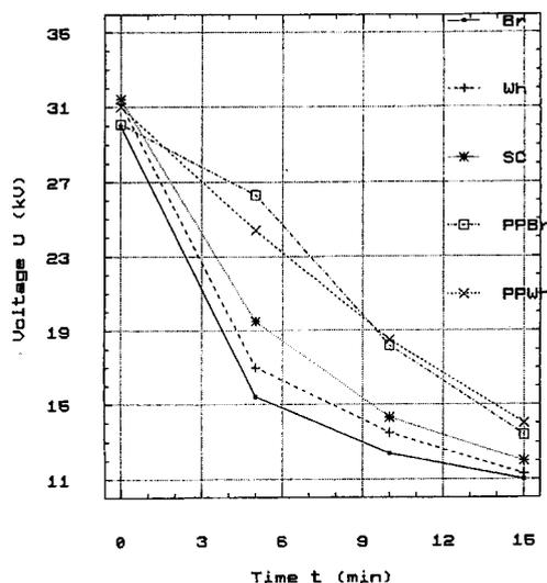
Fig. 2. AC flashover voltage as a function of wetting time in fog chamber: Br - brown glaze; Wh - white glaze; SC - fluorourethane coating; PPBr, PPWh - plasma treated brown and white glaze respectively.
