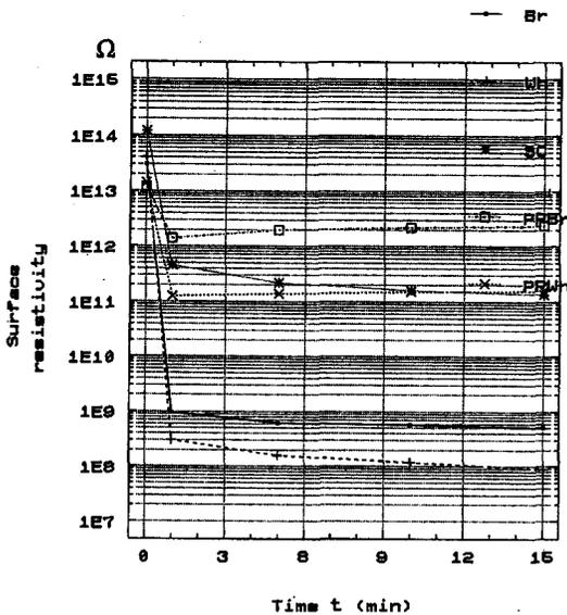
Fig. 4 Surface resistivity versus time of wetting in fog chamber.
