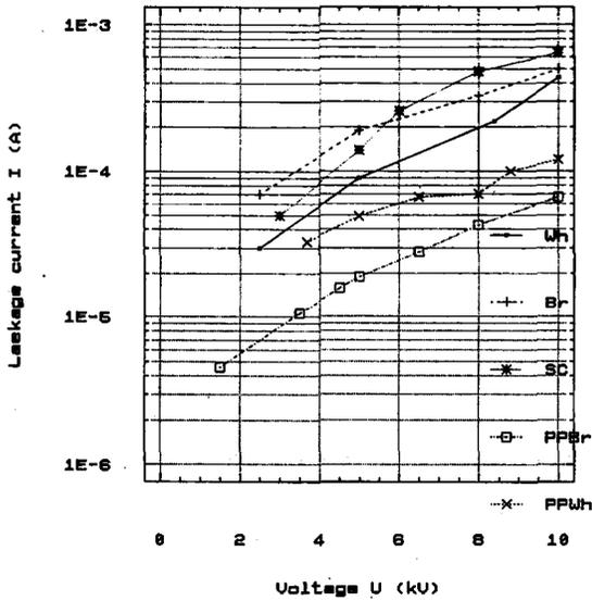
Fig. 3. Leakage current versus DC voltage after 15 min. wetting.
