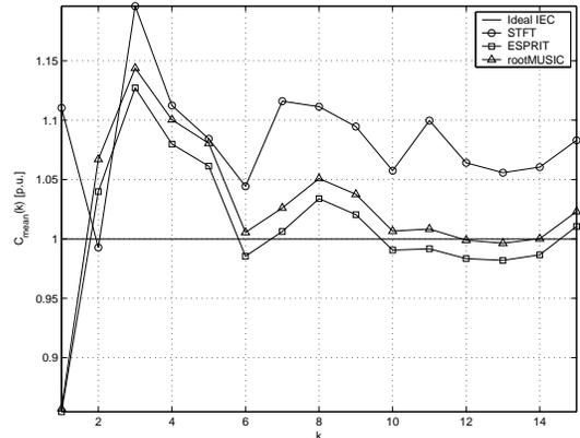
Figure 5. Progressive average of the fifth harmonic subgroup of the voltage.
