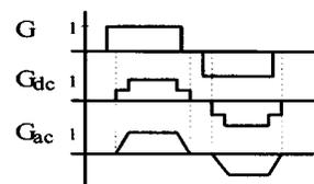
Fig. 5. Voltage and current transfer functions with firing angle variation and commutation overlap.
