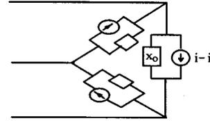
Fig. 7. The converter Norton-equivalent circuit.
