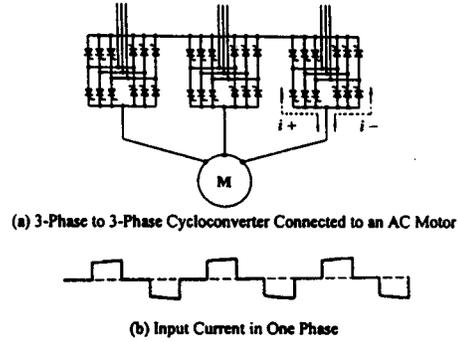
Fig. 15. A 3-phase to 3-phase cycloconverter and its input phase current.
