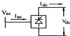
Fig. 4. A simplified schematic converter model.
