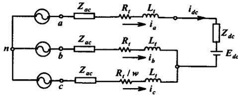
Fig. 9. The simplified converter circuit.
