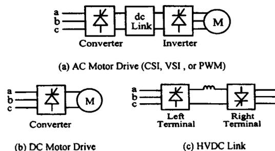
Fig. 2. Typical configurations of AC/DC motor drives and the HVDC link.
