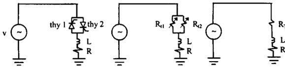
Fig. 14. The equivalent circuit for the TCR.
