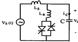
Fig. 13. The simplified single-phase SVC circuit.
