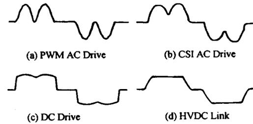
Fig. 3. Typical converter input current waveforms of AC/DC motor drives and the HVDC link.
