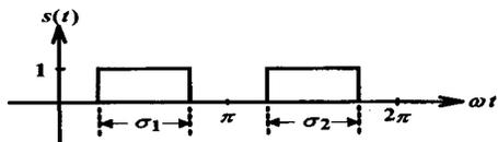
Fig. 12. The TCR thyristor switching function.
