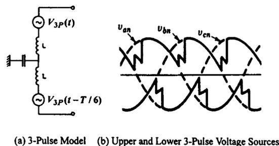
Fig. 8. The six-pulse converter modeled with two 3-pulse voltage sources.
