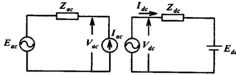
Fig. 6. Converter AC- and DC-side harmonic Thévenin equivalent circuits.
