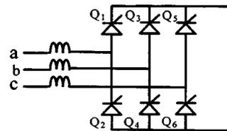
Fig. 1. The six-pulse line-commutated converter.
