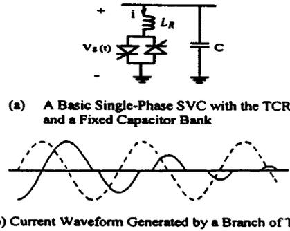
Fig. 10. The SVC configuration and typical TCR current waveform.
