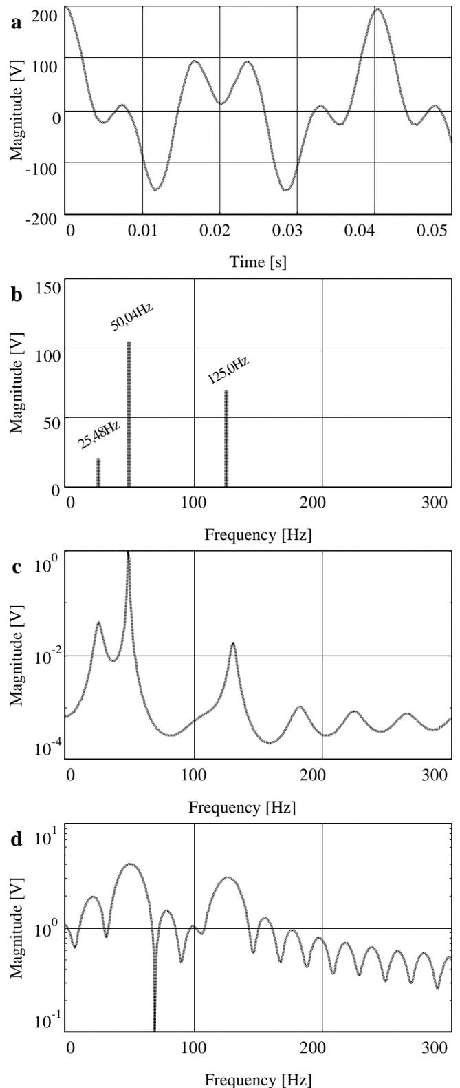
Fig. 1. Voltage waveform at the output of a simulated DC arc furnace power supply installation (a); investigation results: Prony,  $M=30$  (b); min-norm (c); FFT (d);  $f_p=2000$ Hz,  $N=100$ .
