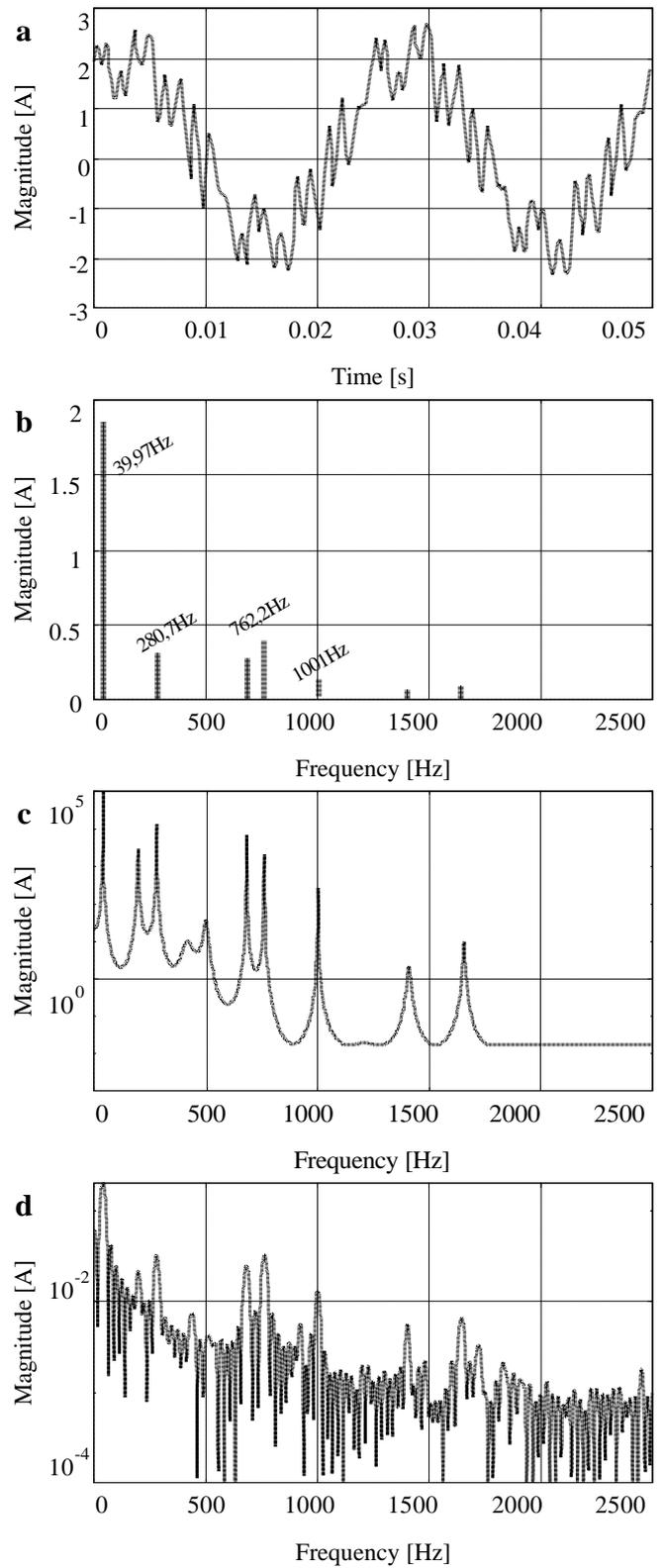
Fig. 3. Current waveform at the output of a real frequency converter (a); investigation results: Prony  $N=200, M=80$  (b); min-norm  $N=100$  (c); FFT  $N=200$  (d),  $f_p=5000\text{Hz}$ .
