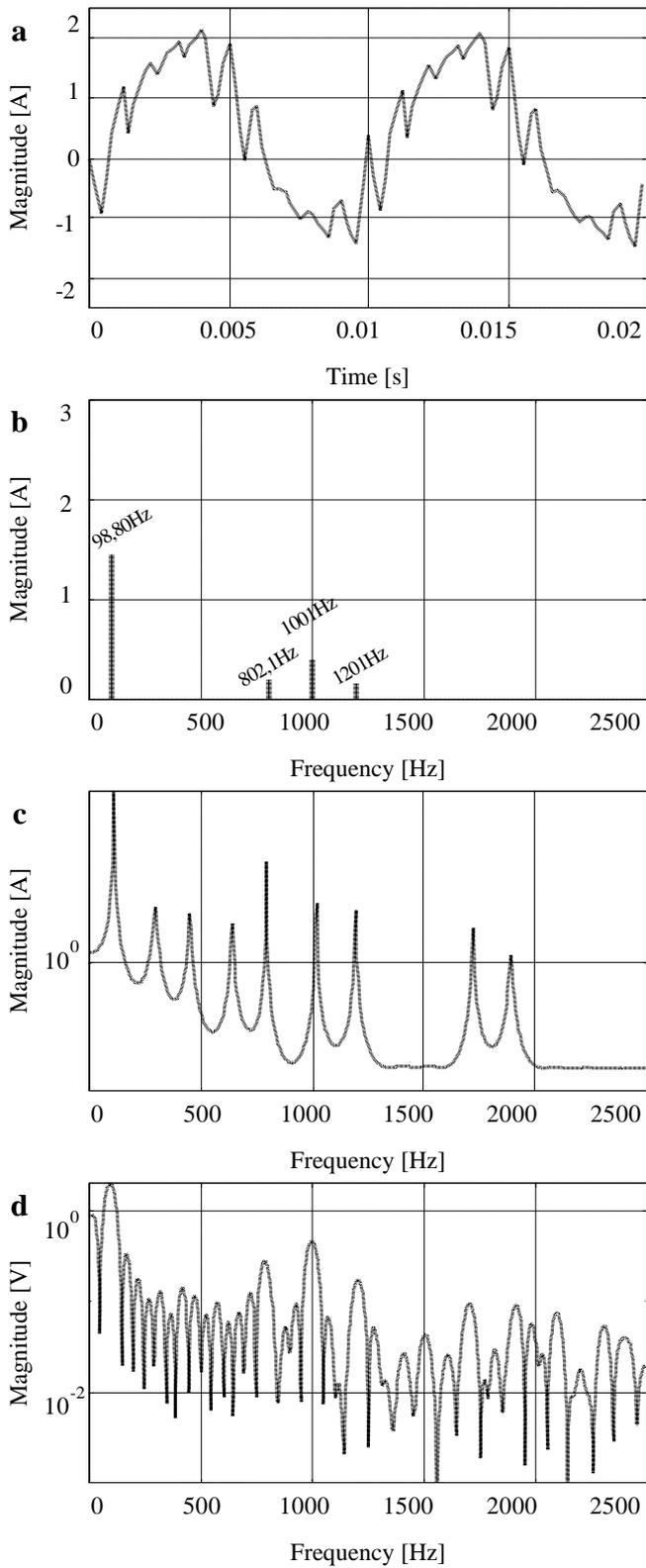
Fig. 2. Current waveform at the output of a simulated frequency converter (a); investigation results: Prony  $N=80, M=40$  (b); min-norm  $N=100$  (c); FFT  $N=80$  (d);  $f_p=5000\text{Hz}$ .
