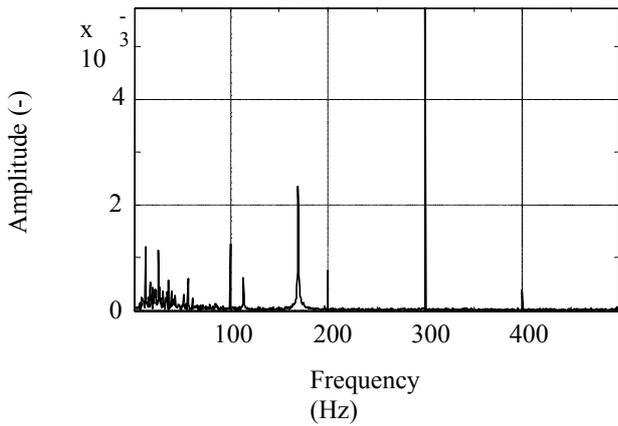
Fig. 2. Power spectrum of the current in the supply system with a filter.
