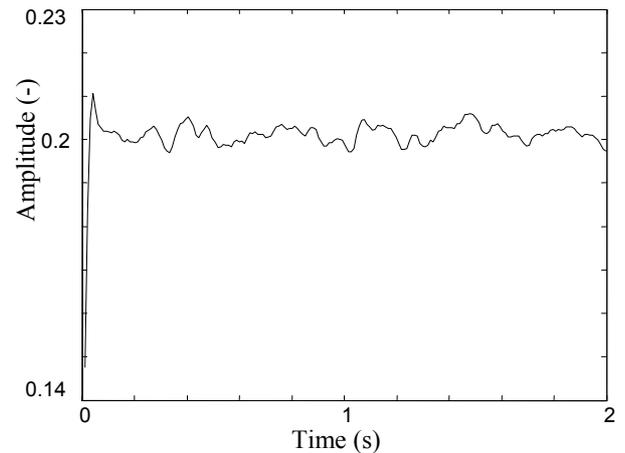
Fig. 9. Time-amplitude representation of the  $\sim 300$  Hz component in the system without filter, estimated by ESPRIT method.
