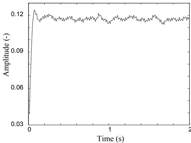
Fig. 7. Time-amplitude representation of the  $\sim 170$  Hz component in the system with a filter, estimated by ESPRIT method.
