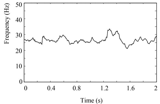
Fig. 6. Time-frequency representation of the subharmonic in the system with a filter, estimated by ESPRIT method.
