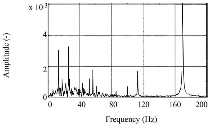
Fig. 3. Power spectrum of the current in the supply system without filter.
