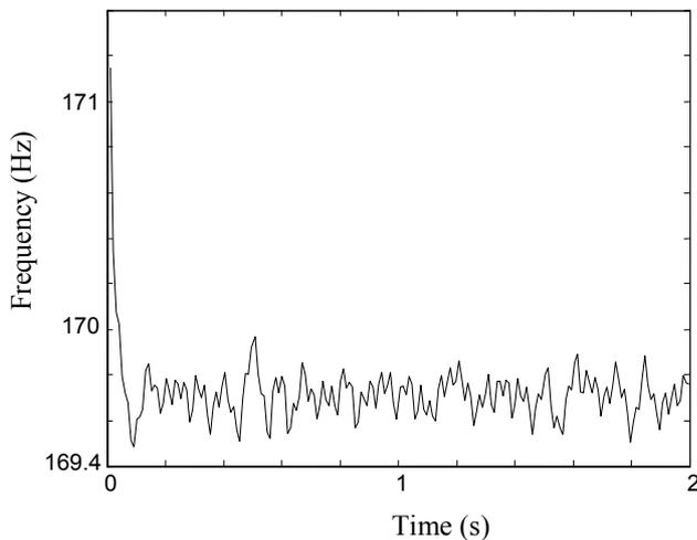
Fig. 8. Time-frequency representation of the  $\sim 170$  Hz component in the system with a filter, estimated by ESPRIT method.
