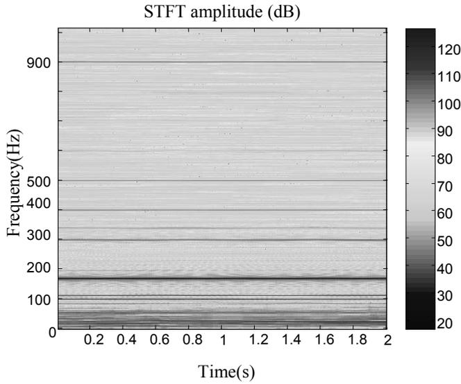
Fig. 1. Short-Time Fourier Transform of the supply current without filter.
