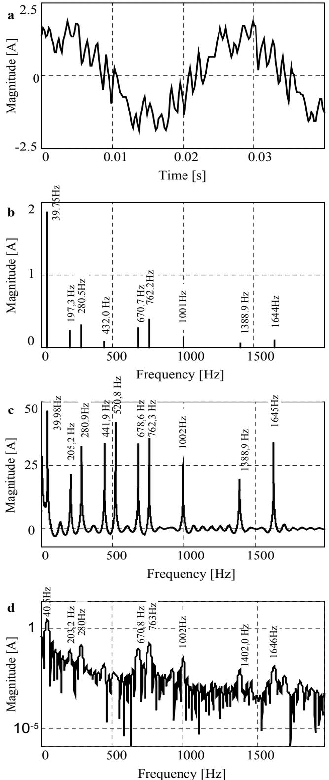
Fig. 2. Current waveform at the output of a real frequency converter (a); investigation results: Prony  $N=200, M=80$  (b); min-norm  $N=100$  (c); FFT  $N=200$  (d),  $f_p=5000\text{Hz}$
