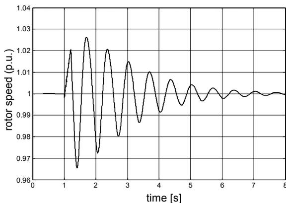
Fig. 4 Rotor speed of the generator during out-of-step operation (p.u.)
