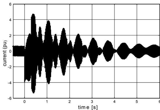
Fig. 3 Current waveform at the generator output. Duration of the fault 300 ms.
