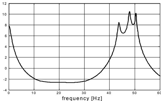
Fig. 5. Stator current spectrum of the signal in Fig. 3, for  $t=2$  s after fault incipience. Detected signal components with frequencies: 43.75, 47.95 and 50.49 Hz.
