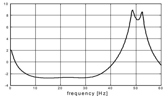
Fig. 6. Stator current spectrum of the signal in Fig. 3 for  $t=4$  s after fault incipience. Detected signal components with frequencies: 48.63 and 52.54 Hz.
