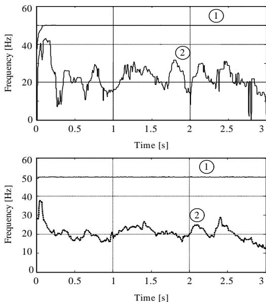
Fig. 6. Time frequency characteristics of the 2 voltage components in the range 0-50 Hz Hz, Prony method (upper fig.), root-MUSIC method (lower fig.).
