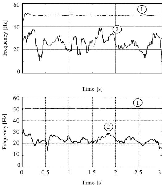
Fig. 5. Time frequency characteristics of the 2 current components in the range 0-50 Hz, Prony method (upper fig.), root-MUSIC method (lower fig.).
