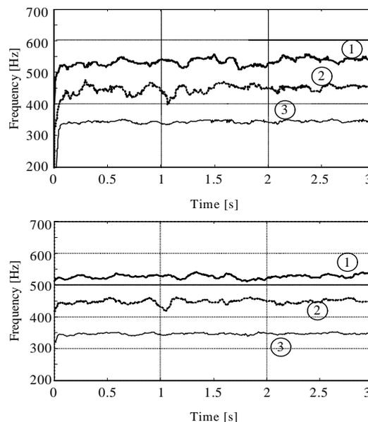
Fig. 3. Time frequency characteristics of the 3 current components in the range 300-500 Hz: Prony method (upper fig.), root-MUSIC method (lower fig.)
