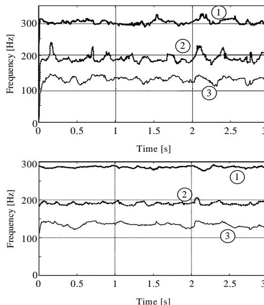
Fig. 4. Time frequency characteristics of the 3 voltage components in the range 100-300 Hz, Prony method (upper fig.), root-MUSIC method (lower fig.)
