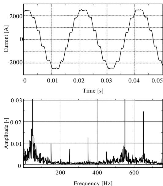
Fig. 2. Current waveform at MV busbar of the dc arc furnace from Fig. 1 (upper fig.) and its power spectrum (lower fig.).
