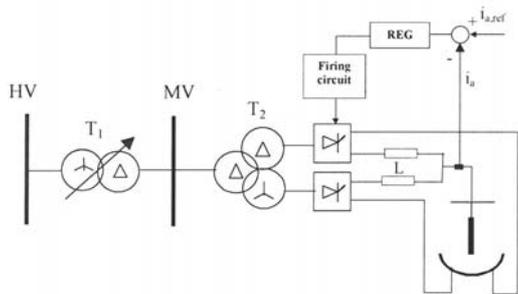
Fig. 1. Modeled DC arc furnace plant
