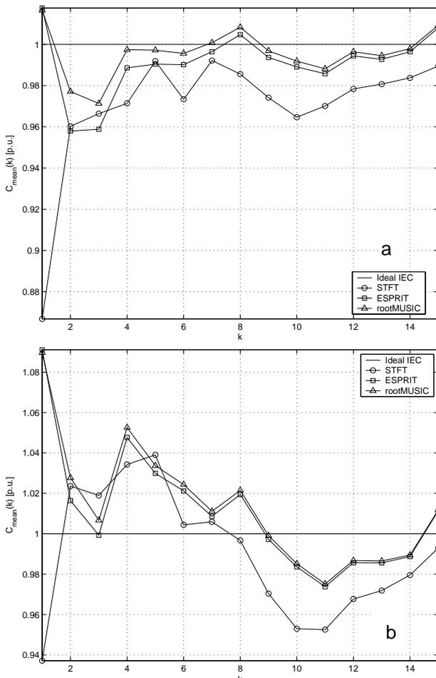
Fig.5. Progressive average of the 11<sup>th</sup> (a) and 13<sup>th</sup> (b) harmonic component of the current.
