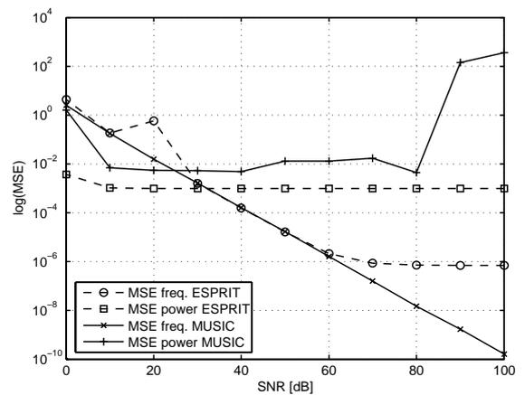
Fig.1. MSE of frequency and power estimation depending on SNR.
