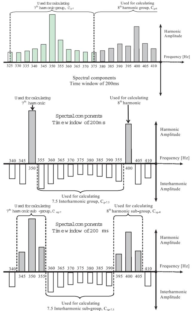
Fig. 4. Examples of harmonic (↑) and interharmonic (↓) (sub)groups according to IEC Standard drafts 61000-4-7 and 61000-4-30.
