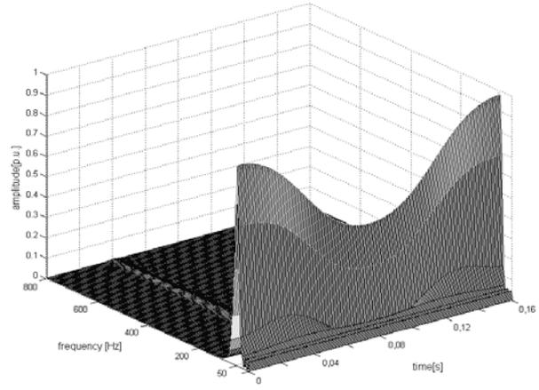
Fig.1. Time-frequency representation of a 50% voltage sag and  $k=1.0$  using the S-transform.
