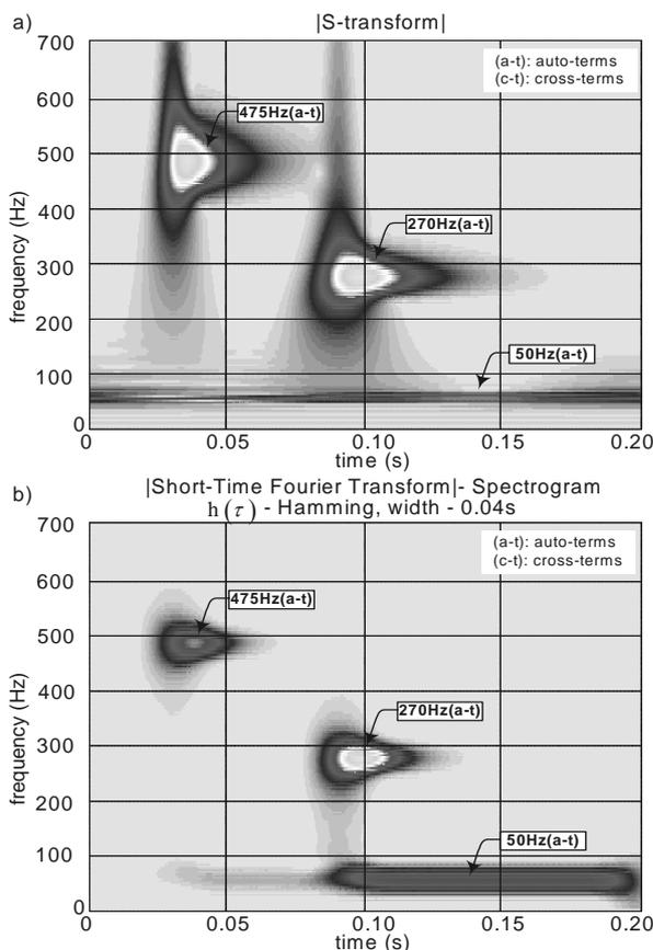
Fig. 7. Comparison of S-transform representation and STFT spectrum of the waveform.
