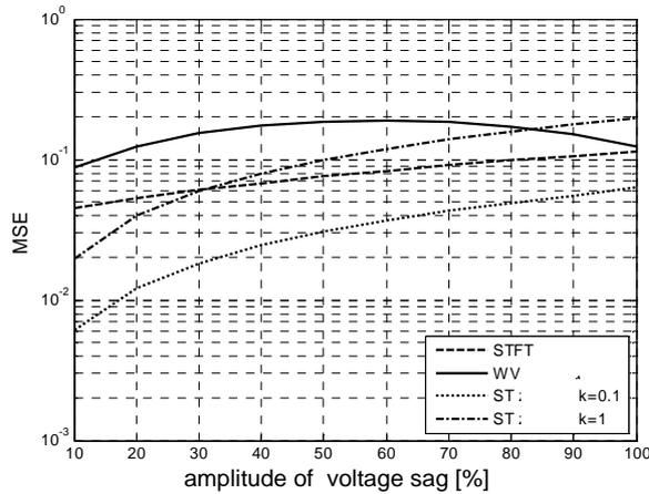
Fig. 3. Representation error for varying amplitude of voltage sag.
