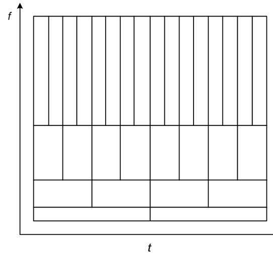
Fig. 5. Frequency-dependent resolution of the S-transform.
