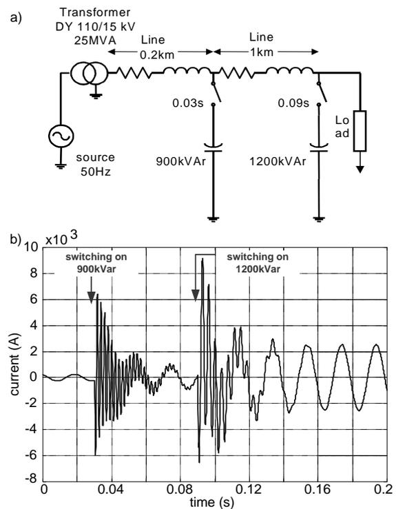
Fig. 6. a) One-phase diagram of the simulated distribution system. b) Voltage waveform at the beginning of the feeder.
