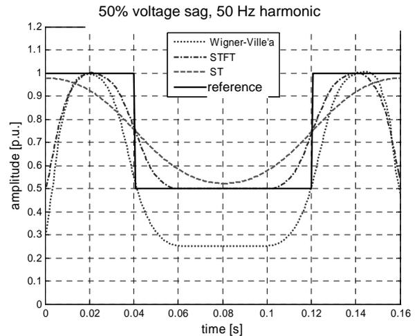
Fig. 2. Representation of the reference signal using the S-transform (ST) for  $K=1$ , the Short-Time Fourier Transform (STFT) – window length = 0.04 s and the Wigner-Ville Transform with smoothing window length of 0.04s – of the test waveform: 50% voltage sag.
