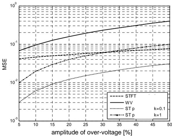
Fig. 4. Representation error for varying amplitude of over-voltage.
