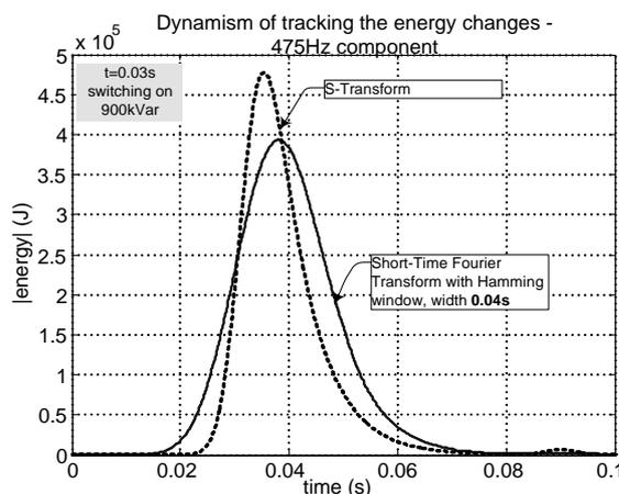
Fig. 8. Comparison of tracking capabilities of dynamic amplitude changes of the 475 Hz components.
