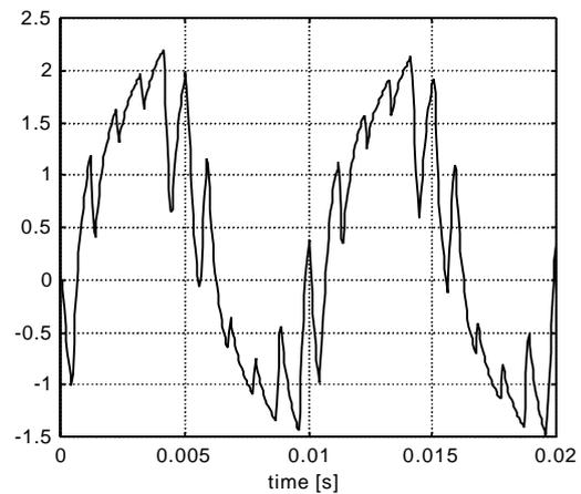
Fig. 2. Current waveform at the output of a simulated frequency converter,  $f = 100$  Hz.
