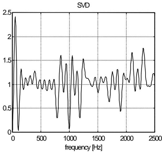
Fig. 3. Magnitude characteristics of the signal in Figure 2 calculated by the MUSIC ( $n=100$ ) and SVD ( $l=254, n=260$ ) method.
