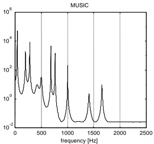
Fig. 5. Magnitude characteristic SVD method and by the MUSIC method of the signal in Fig. 4,  $l=70, n=100$ .
