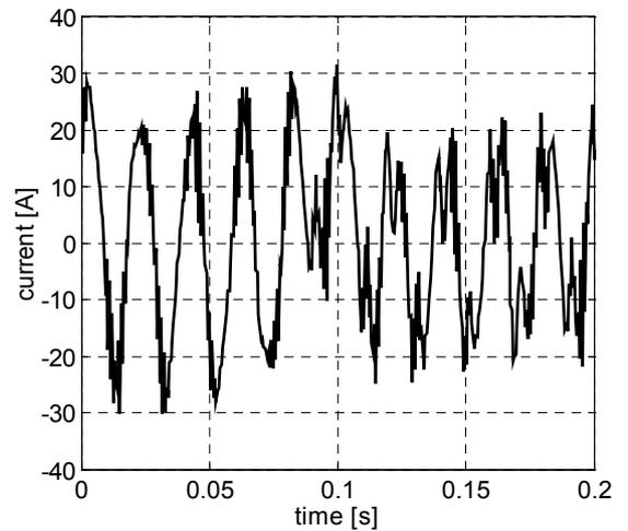
Figure 2. Inverter output current in the phase A. Fault occurs at the time point  $t=0.1$  s
