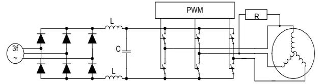
Figure 1. Simplified scheme of the simulated converter configuration. R – resistance of the short-circuit.
