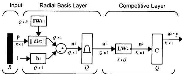
Figure 3. Architecture of the probabilistic neural network [5].
