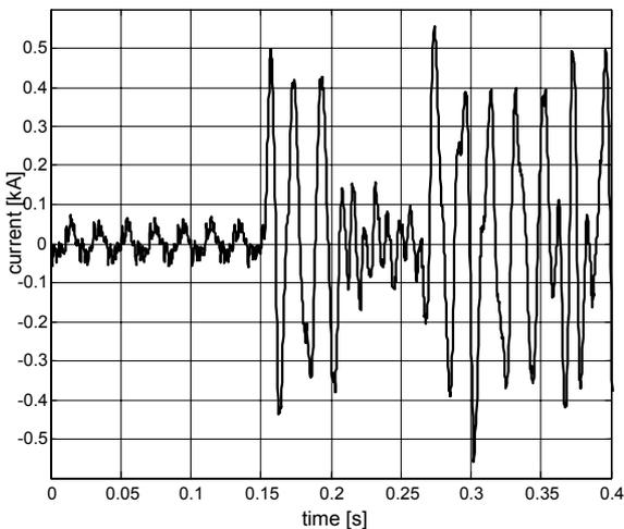
Fig. 9. Signal recorded at the output of an AC arc furnace power supply installation
