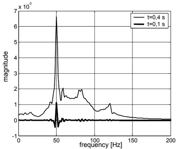
Fig. 11. Cross-sections of the Wigner-Ville representation of the signal in Fig. 7 for time slices  $t=0,1$  and  $0,4$  s
