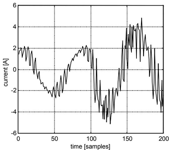
Fig. 3. Current waveform (phase R) at the motor input during a short circuit. Fault occurs after the 100<sup>th</sup> sample.
