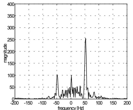
Fig. 7. Estimated WVD of the space-phasor of the fault signal during the motor lead to ground short-circuit in the converter drive (high short-circuit resistance).
