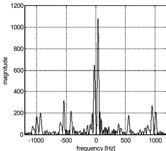
Fig. 5. Estimated WVD of the space-phasor (signal in figure 3), at the time point  $t=0.06$  s. (during the fault).
