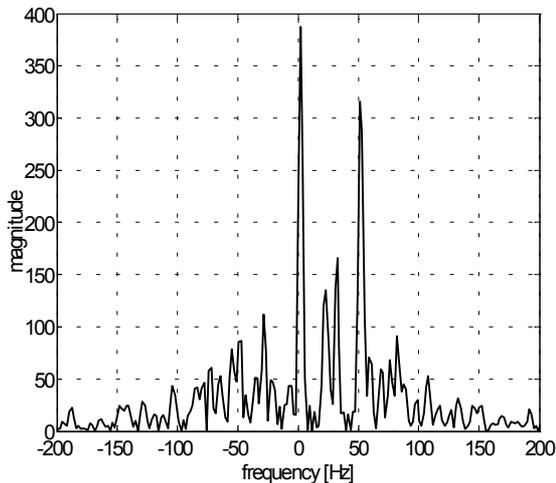
Fig. 8. Estimated WVD of the space-phasor of the fault signal during the motor lead to ground short-circuit in the converter drive (low short-circuit resistance).
