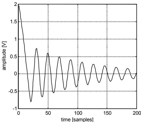
Fig. 1. Voltage waveform in faulted phase during single line to ground short circuit.
