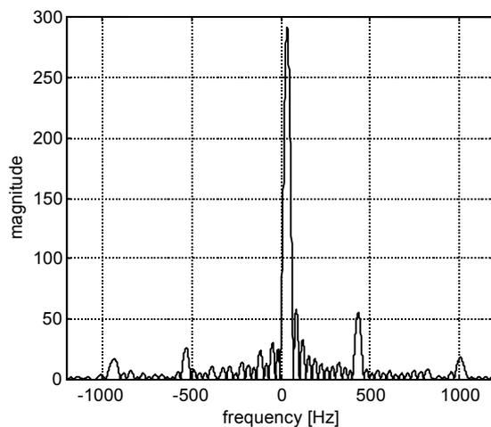
Fig. 4. Estimated WVD of the space-phasor (signal in Fig. 3), at the time point  $t=0.015$  s. (before the fault).
