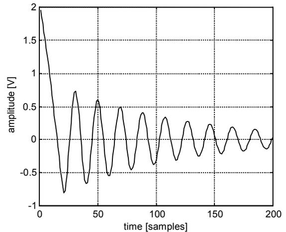
Fig. 7. Voltage waveform (faulted phase) during single line to ground short circuit. Fault occurs after the 20<sup>th</sup> sample.
