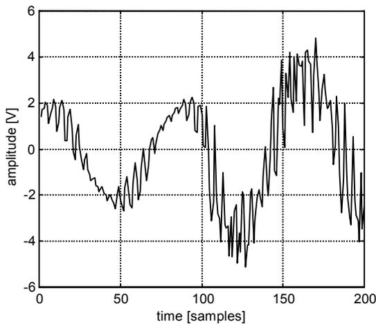
Fig. 1. Voltage waveform (phase R) at the motor input during a short circuit. Fault occurs after the 100<sup>th</sup> sample.
