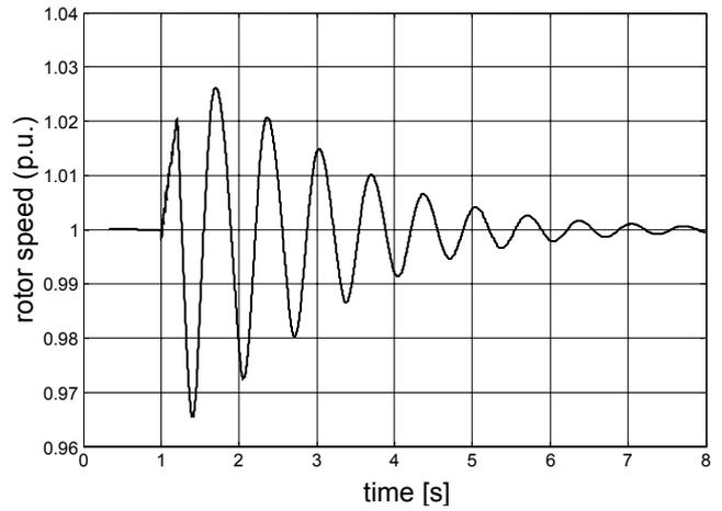
Fig. 6 Rotor speed of the generator during fault (p.u.)
