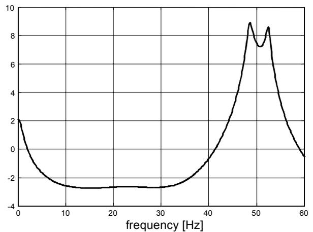
Fig. 8. Stator current spectrum of the signal in Fig. 5 for  $t=4$  s after fault incipience. Detected signal components with frequencies: 48.63 and 52.54 Hz.
