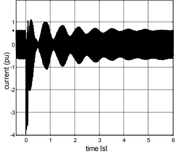
Fig. 2. Current waveform at the generator output. Duration of the fault 100 ms.
