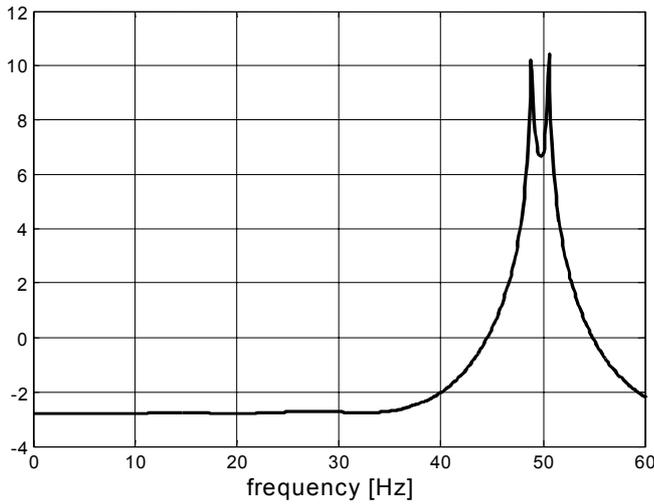
Fig. 4. Stator current spectrum of the signal in Fig. 2, for  $t=4$  s after fault incipience. Detected signal components with frequencies: 48,83 and 50,68 Hz.
