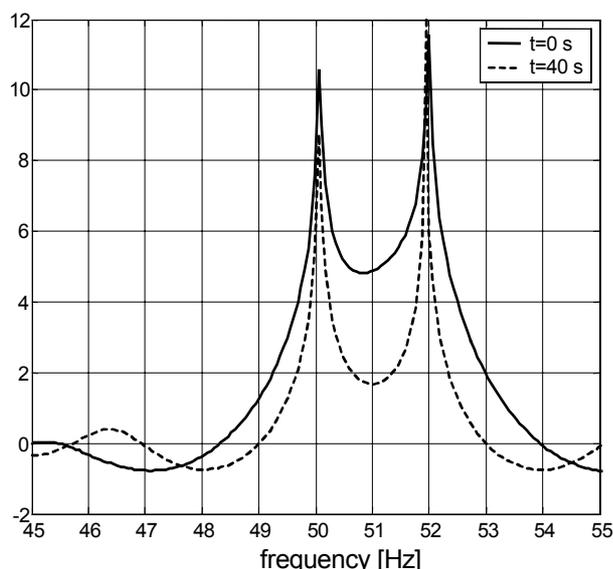
Fig. 10 Stator current spectrum of the signal in Fig. 8. **Solid line** – at the beginning of the asynchronous running: detected components 50, 52 Hz; **Dash line** – after 40 s of the asynchronous running: detected components 50, 51,8 Hz.
