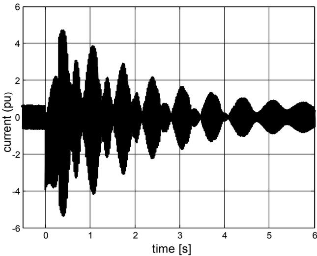
Fig. 5 Current waveform at the generator output. Duration of the fault 300 ms.
