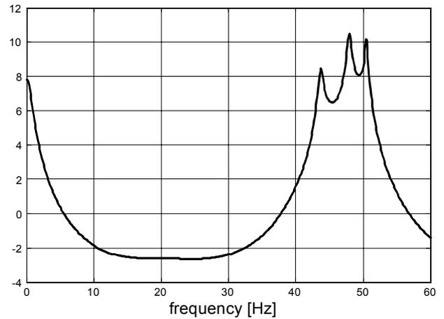
Fig. 7. Stator current spectrum of the signal in Fig. 5, for  $t=2$  s after fault incipience. Detected signal components with frequencies: 43.75, 47.95 and 50.49 Hz.
