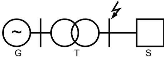
Fig. 1. Modelled power system.
