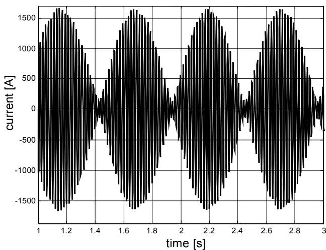
Fig. 9 Current waveform at the generator output, recorded at the physical model..
