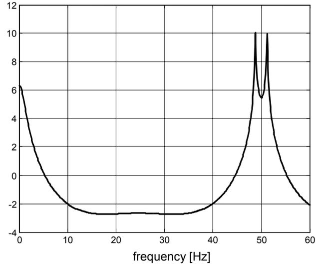
Fig. 3. Current spectrum of the signal in Fig. 2, for  $t=2$  s after the fault incipience. Detected signal components with frequencies: 48,73 and 51,27 Hz.
