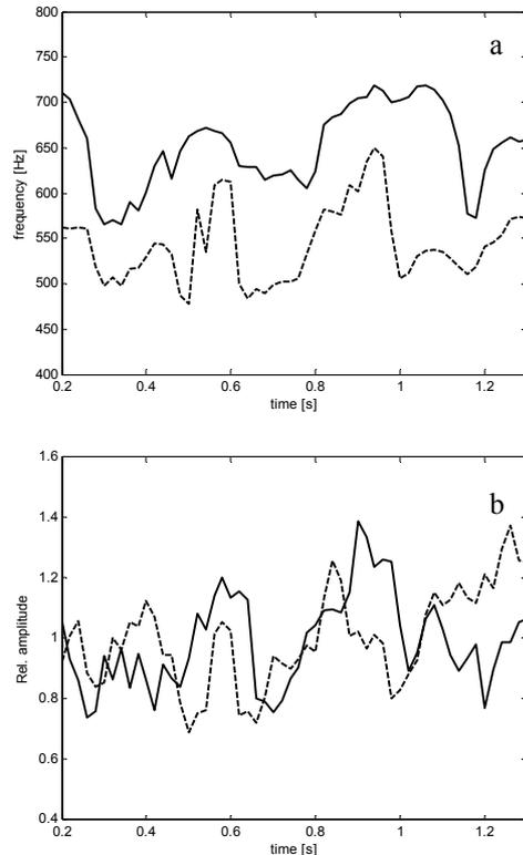
**Figure 6:** Time-varying frequency (a) and relative amplitude (b) (relative to the mean amplitude over the analysis interval) of MV voltage with active filters at 11<sup>th</sup> and 13<sup>th</sup> harmonic.
