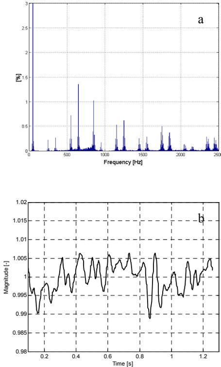
**Figure 4:** Voltage fundamental component at the DC arc furnace with Active Filter: a) spectrum (FFT on 1 s window); b) magnitude versus time (PRONY representation for 100 samples in window analysis, sampling frequency 5000 Hz)
