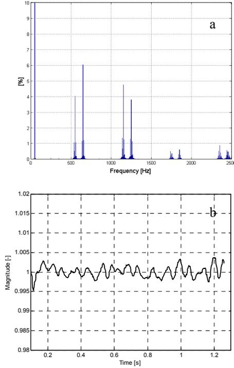
**Figure 3:** Voltage fundamental component at the DC arc furnace with STATCOM: a) spectrum (FFT on 1 s window); b) magnitude versus time (PRONY representation for 100 samples in window analysis, sampling frequency 5000 Hz)
