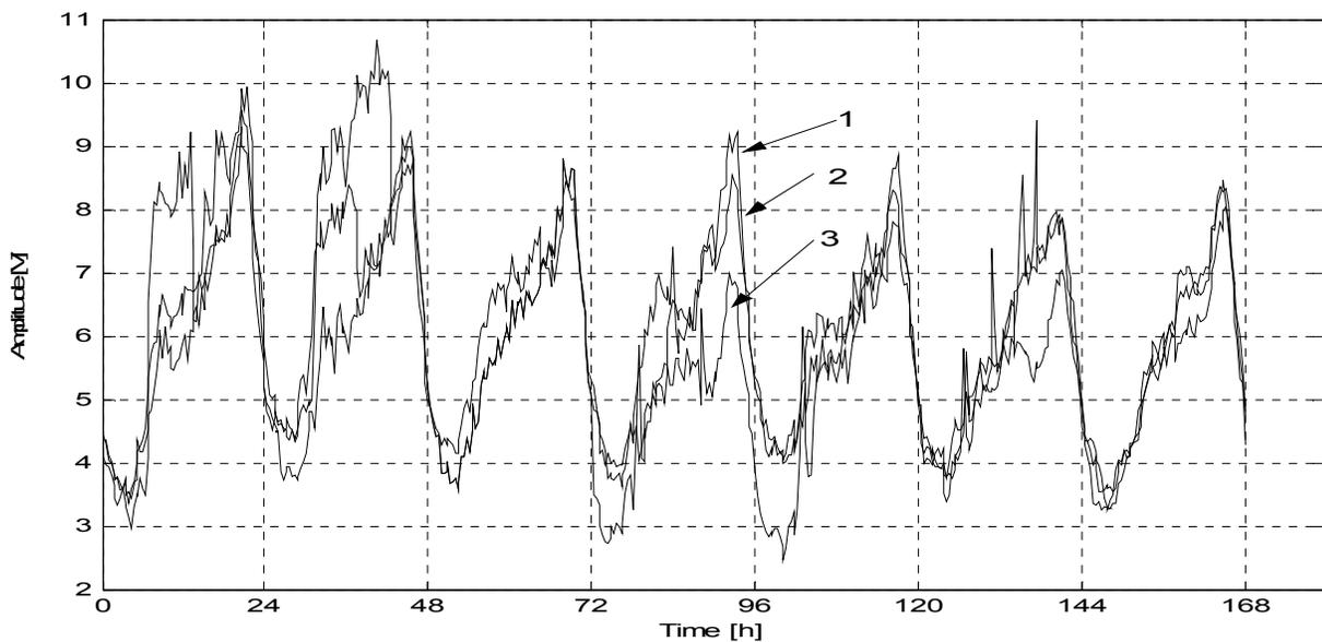
Fig. 2 Time-plot of 5<sup>th</sup> voltage harmonic for three consecutive weeks (1, 2, 3) at PCC 2
