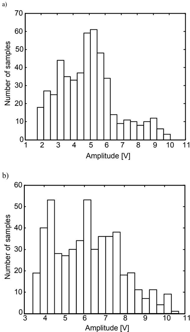
Fig. 5. The 20 bins histogram of 5<sup>th</sup> harmonic voltage for: a) PCC1
