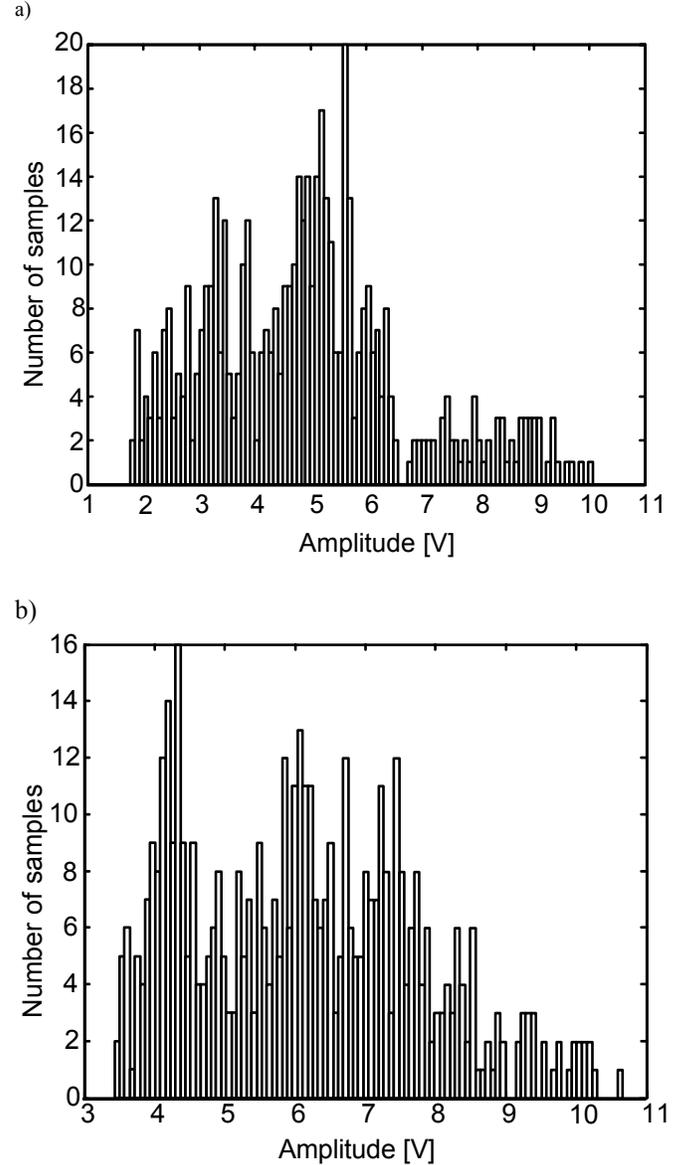
Fig. 5. The 100 bins histogram of 5th harmonic voltage for: a) PCC1 b) PCC2
