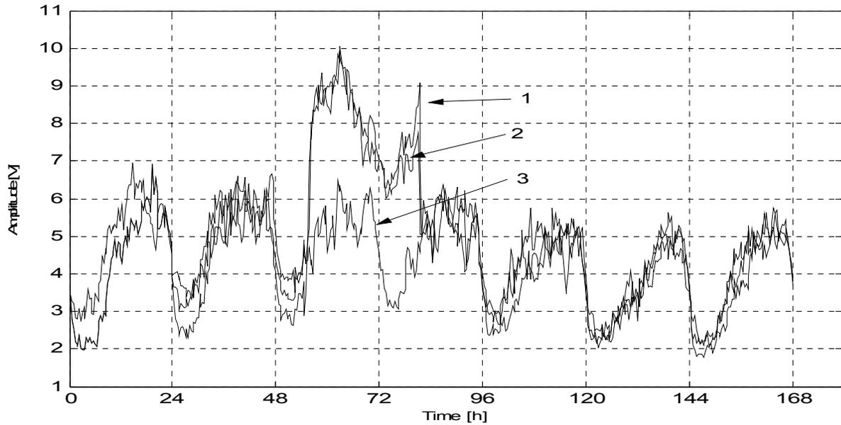
Fig. 1 Time-plot of 5<sup>th</sup> voltage harmonic for three consecutive weeks (1, 2, 3) at PCC 1
