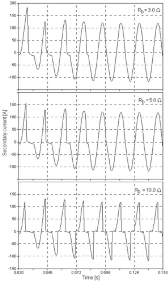
Fig. 4. Distortions in secondary current dependent on the CT burden.
