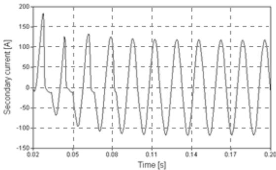
Fig.5. Secondary current for  $X/R = 8$ .
