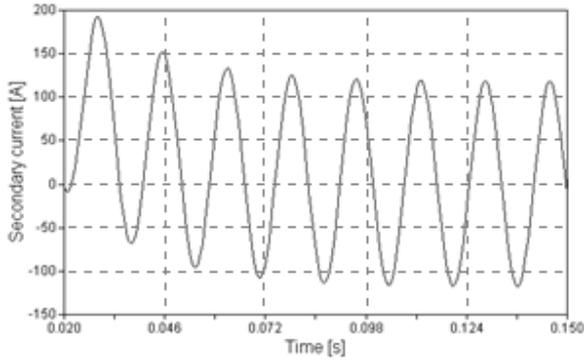
Fig. 3. Undistorted secondary current ( $R_B = 0.3 \Omega$ ).
