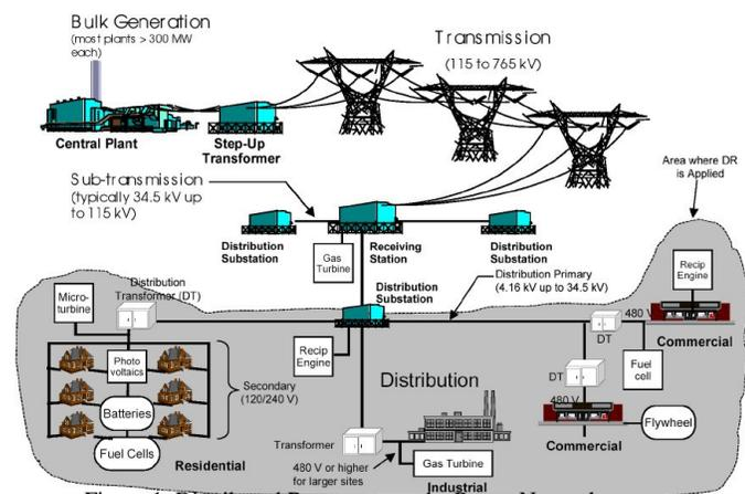
Figure 1, Distributed Resources on the Power Network
