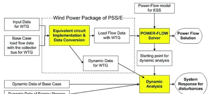
Figure 3. Overview of the implemented WTG/ESS simulation using PSS/E
