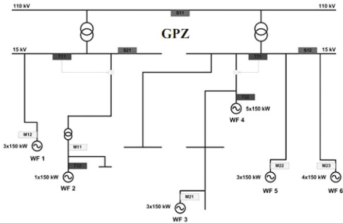
Figure 2. Scheme of analyzed medium voltage network
