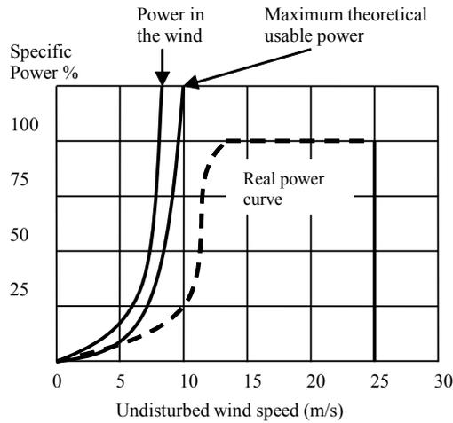
Figure 1. Power output in relation to wind speed
