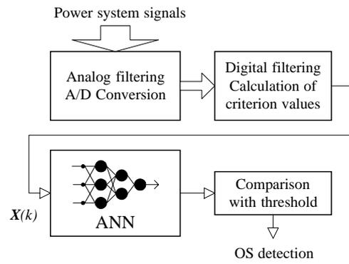
Fig. 7. Neural OS protection arrangement.
