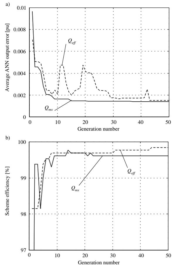
Fig. 9. Optimisation results: a) mean square error, b) recognition efficiency.
