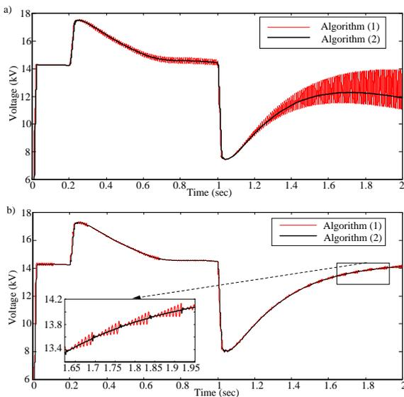
Fig. 4. Amplitude estimation with algorithms: a) non-adaptive, b) with adaptation.
