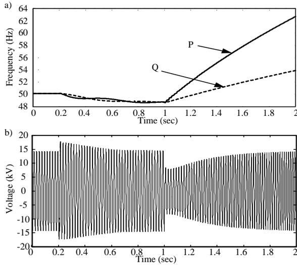
Fig. 3. Transient signals picked up at busbar GP: a) rotor's speed of generators P and Q, b) phase A voltage.
