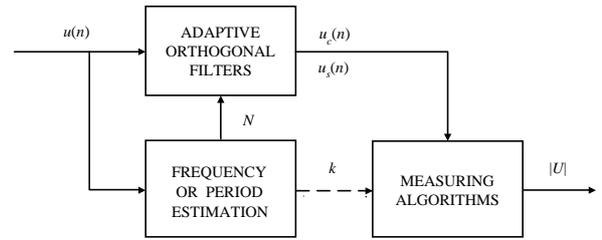
Fig. 1. Block scheme of the amplitude measurement with adaptive orthogonal filters.
