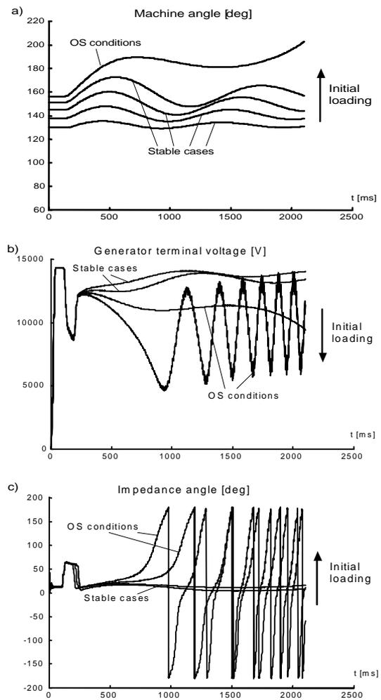
Fig. 2. Exemplary machine signals for stable cases and OS conditions: a) machine angle, b) generator terminal voltage, c) impedance vector angle.
