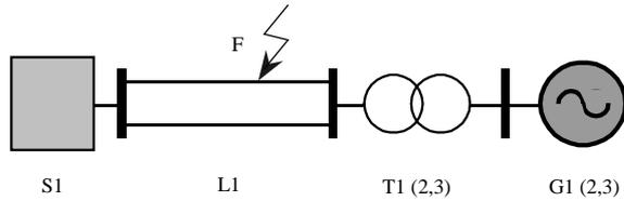
Fig. 1. Fragment of power system modelled in EMTP/ATP.
