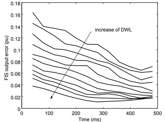
Fig. 6. Average FIS output error vs. time (DWB location).
