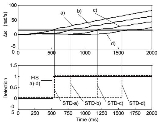
Fig. 9. Response of FIS-based (FIS) and standard (STD) OS protection for chosen simulation cases: a) severe fault by high pre-fault load, b) middle pre-fault load, c) low pre-fault load, d) case with autoreclosure.
