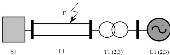
Fig. 5. Test power system modeled in ATP.
