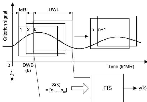
Fig. 4. Data capturing with sliding data window.
