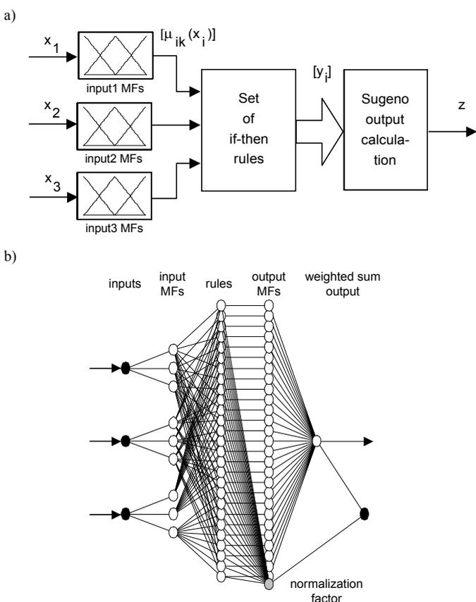
Fig. 2. FIS studied: a) general structure, b) adaptive network representation.
