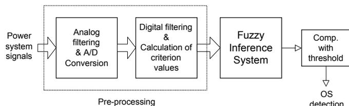
Fig. 3. General structure of the FIS-based OS protection.
