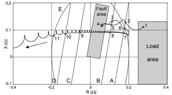
Fig. 8. Standard impedance-based OS detection scheme.
