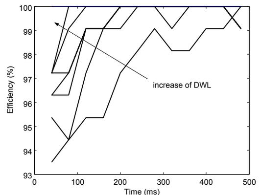
Fig. 7. Average FIS operation efficiency vs. time (DWB location).
