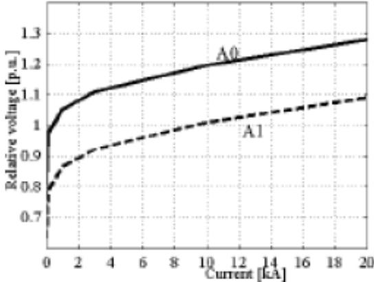
Figure 3. Characteristics of nonlinear elements  $A_0$ ,  $A_1$  of IEEE arrester model
