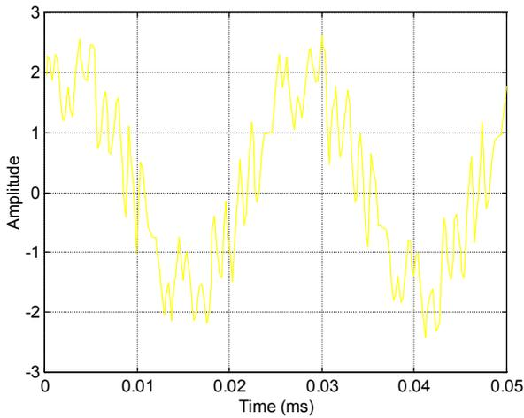
Fig.3 Current waveform at the output of frequency converter.
