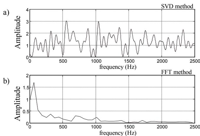
Fig.4 Magnitude characteristic of  $\mathbf{H}(z)$  at the SVD - method and the FFT method of the signal in Fig.3,  $l=70$ ,  $n=80$ .
