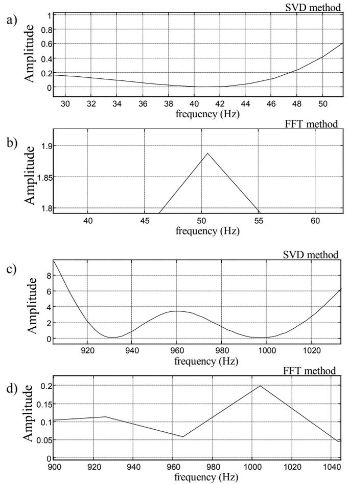
Fig.5 Magnitude characteristic of  $\mathbf{H}(z)$  at the SVD - method (a, c) and the FFT method (b, d) of the signal in Fig.3,  $l=70$ ,  $n=100$ . a,b - enlargement for frequency estimation of the fundamental harmonic. c,d- enlargement for frequency estimation of higher harmonics.
