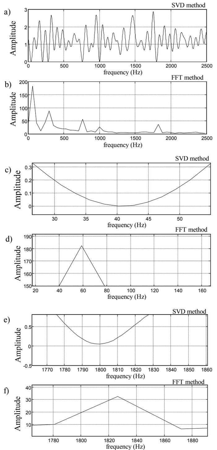
Fig.2 Magnitude characteristic of  $\mathbf{H}(z)$  at the SVD - method (a, c, e) and the FFT method (b, d, f) of the signal in Fig.1,  $n = 85$ .
