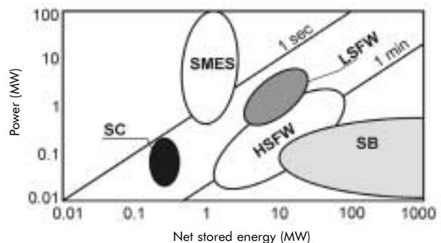
Figure 17 - Power v energy characteristics of different energy storage systems [7]
