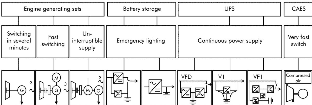
Figure 3 - Types of reserve power supply devices
