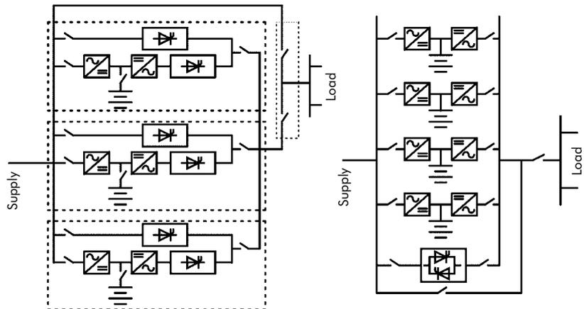
Figure 15 - Systems of UPS devices in parallel operation
