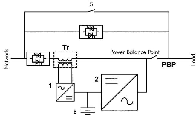
Figure 10 - The block diagram of the Delta type UPS
