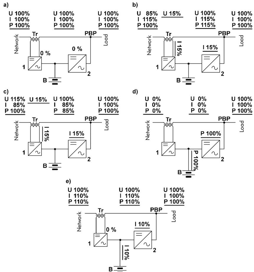
Figure 11 - Illustration of various operation modes of the Delta-UPS
