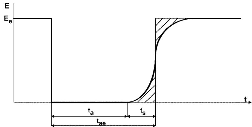
Figure 1 - Production efficiency following a power failure
