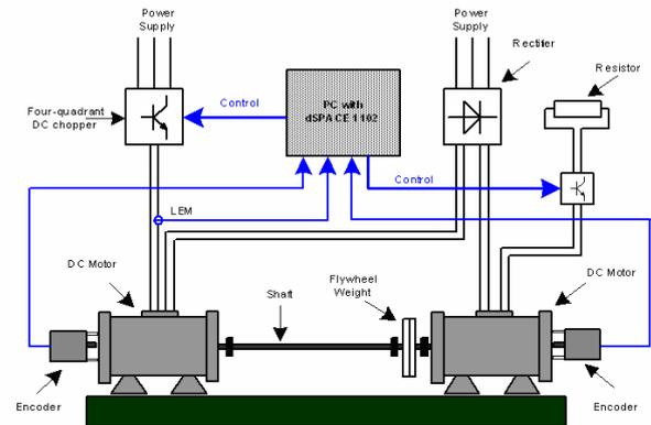
Fig.8. Schematic diagram of the experimental set-up
