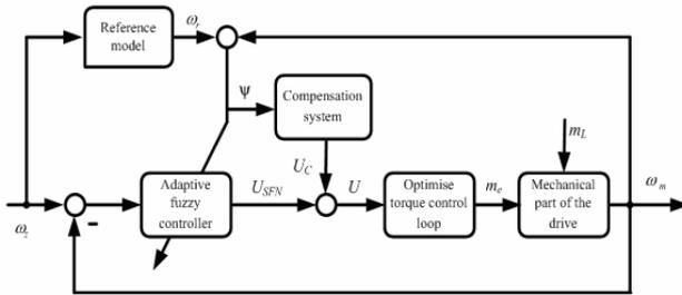
Fig. 2. Structure of the adaptive control system
