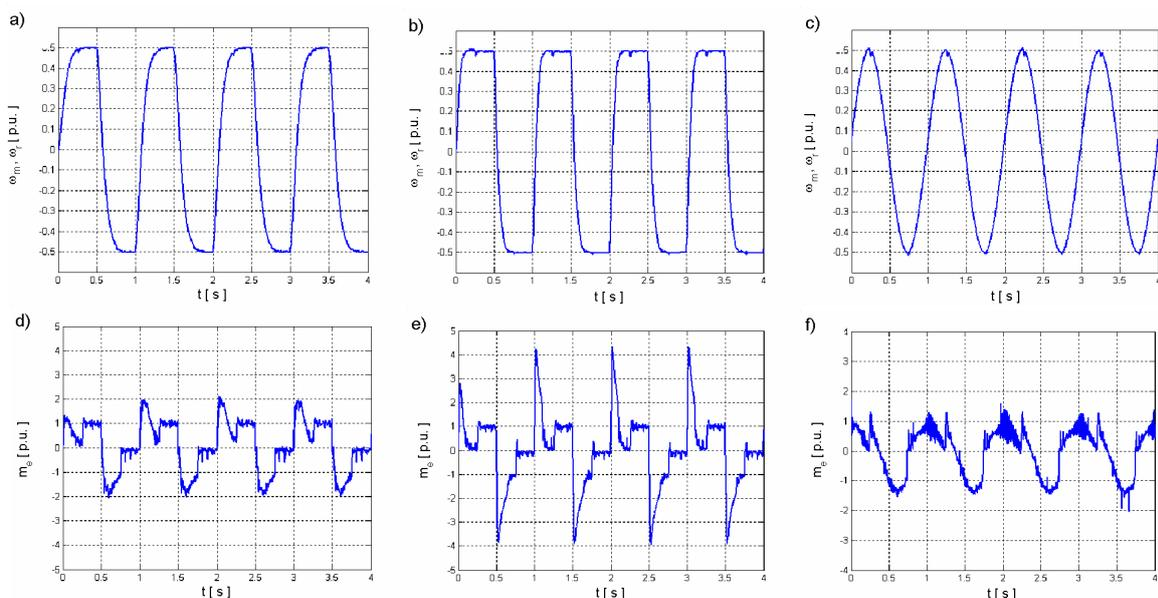
Fig. 9. Experimental transients of the system with nominal parameters: motor and reference speeds (a,b,c), electromagnetic torque (d,e,f), for resonant frequency  $\omega_r=20s^{-1}$ (a,d),  $\omega_r=40 s^{-1}$  (b,e), sinusoidal reference signal (c,f)
