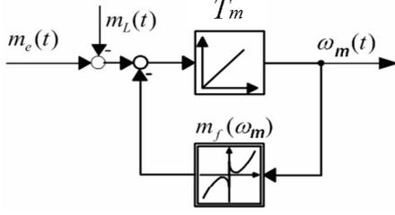
Fig. 1. The block diagram of the one-mass system
