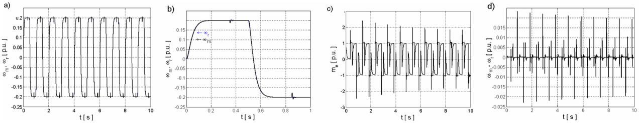
Fig. 5. Transients of the system with nominal parameters, without compensator: motor and reference speed (a,b), electromagnetic torque (c), tracking error (d)
