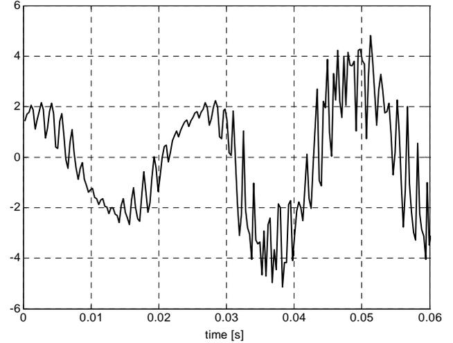
**Figure 12:** Voltage waveform (phase R) at the motor input during a short circuit. Fault occurs after 0.03 s.
