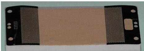
**Figure 1:** The silicone plate contaminated by desert dust and the perforated electrodes.
