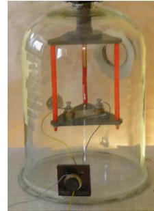
**Figure 2:** The sample inside the glass hygrostat
