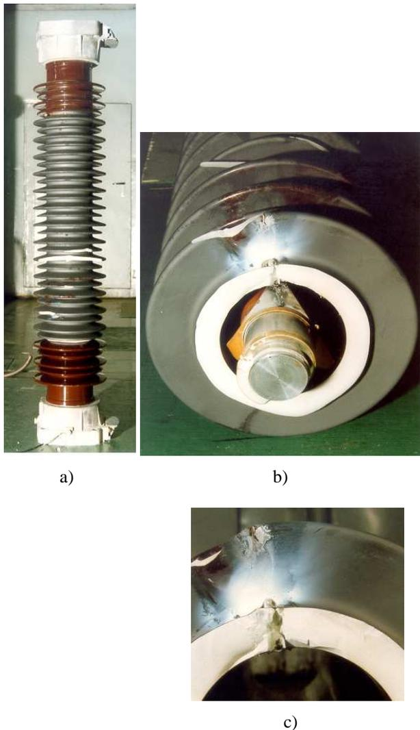
Fig. 2. The damaged surge arrester during an internal arcing test with graphite layer
