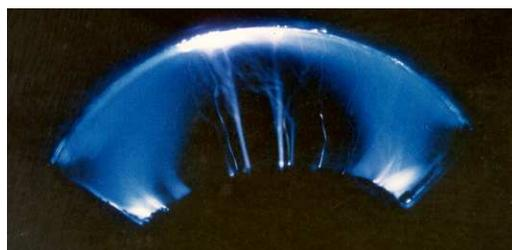
Fig. 1. Intensive partial discharges inside a non-uniformly polluted surge arrester. Test voltage 68 kV.
