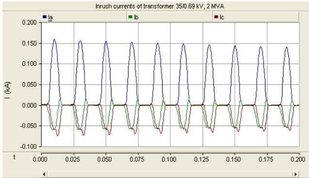
Figure 2: Inrush currents in power transformer 2 MVA during switching on ideal 35 kV source (switching on angle =0°)
