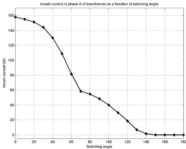
Figure 3: Inrush currents as function of switching-on angle (phase A)
