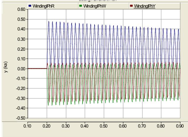
Figure 5: Currents in power transformer 2 MVA during switching on ideal 35 kV source (switching on angle =  $0^\circ$ )
