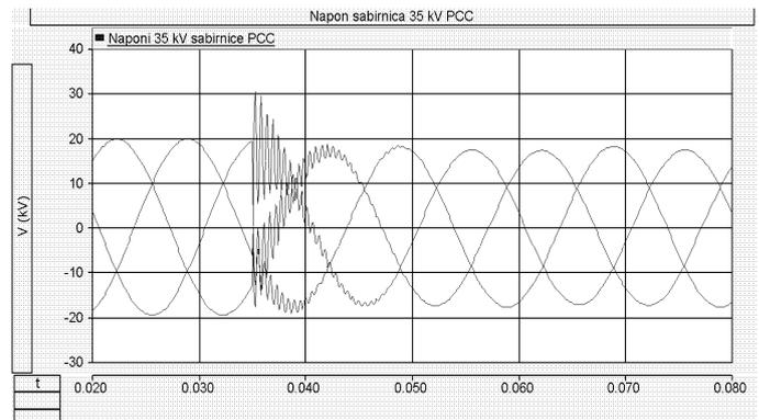
Figure 10. Voltage distortions in the PCC. Simultaneously all twelve block - transformers are switched on
