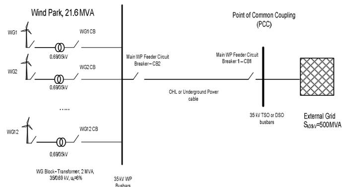
Figure 7. Configuration Scheme of WP connection on Distribution Operator's 35 kV substation
