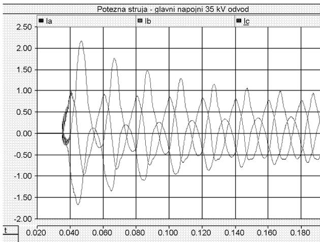
Figure 11. Inrush currents on the main WP feeder . Simultaneously all twelve block – transformers are switched on where 3 of them have remnant magnetism in the core.
