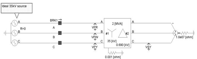
Figure 5: Simulation setup for determining inrush currents in a power transformer 2 MVA during switching on ideal 35 kV source (switching on angle =0°)
