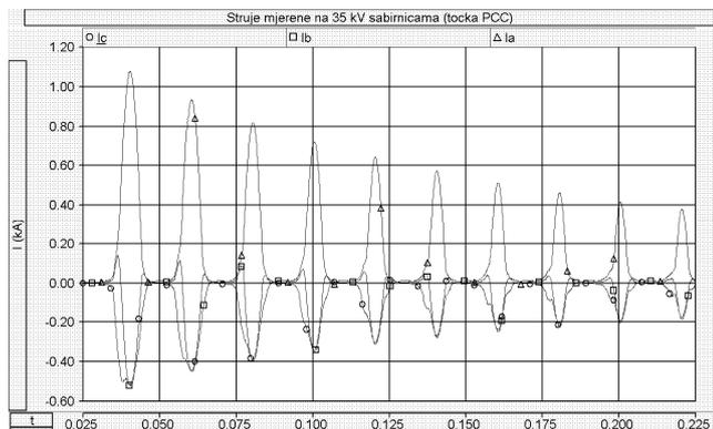
Figure 9. Inrush currents in the main WP feeder when simultaneously all twelve block - transformers are switched on (Main feeder - OHL 150 mm<sup>2</sup>, 5 km length)
