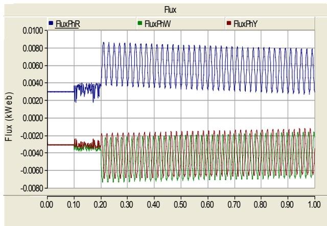
Figure 6: Fluxes in power transformer 2 MVA during switching on ideal 35 kV source (switching on angle =  $0^\circ$ )
