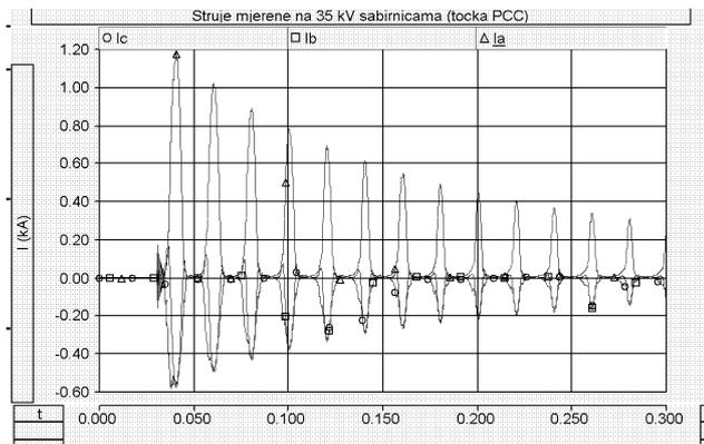
Figure 8. Inrush currents in the main WP feeder when simultaneously all twelve block – transformers are switched on (Main feeder - XLPE cable 150 mm<sup>2</sup>, 5 km length)
