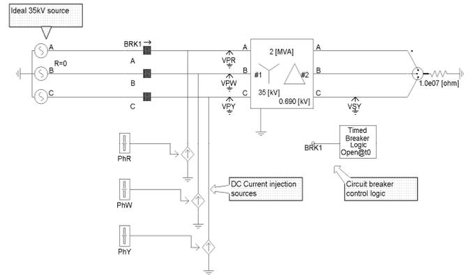
Figure 4: Simulation setup for determining inrush currents in a power transformer 2 MVA during switching on ideal 35 kV source (switching on angle =0°)
