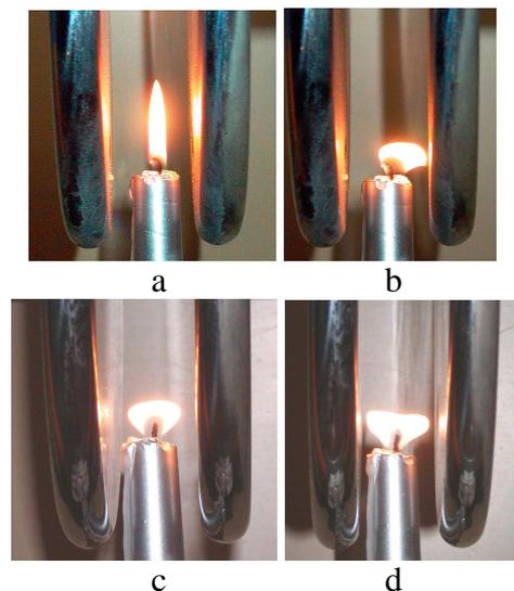
Fig. 1. The flame in an electric field, air gap 3 cm
