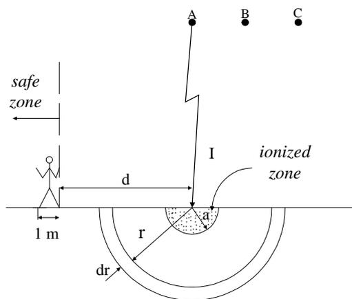
Fig. 4. Step voltage around a flashover point [7]
