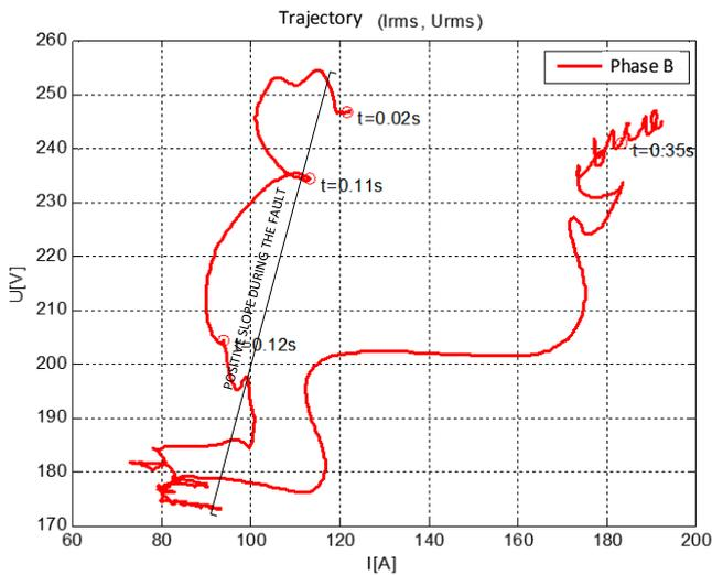
Figure 6. Trajectory (I, U) for the selected phase of the phase voltage dip caused by the lightning stroke.
