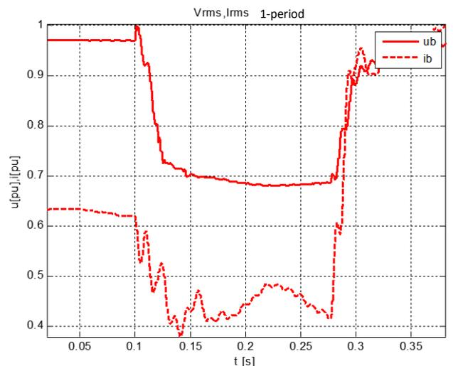
Figure 5. Waveform of 1-periodic normalized RMS voltage and current, at asynchronous generator in SHP connected directly to the low voltage power grid during voltage dip due to an incident from the network occurring at the time of 0,1 s.
