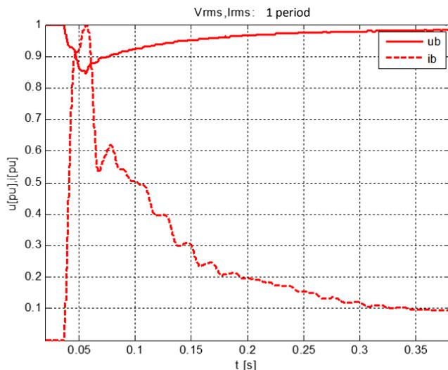
Figure 3. Changes of normalized 1-period RMS voltages and currents caused by the switching-on of the SHP asynchronous generator connected to the grid at the time of 0,05 s.
