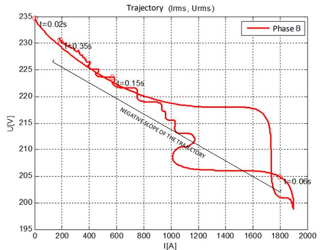
Figure 4. Trajectory (I, U) for the selected phase of the phase voltage dip caused by the switching-on of the SHP asynchronous generator connected to the grid.
