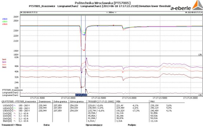
Figure 1. Registrations of RMS values by RecB of selected power quality disturbance seen synchronously in Q1, Q2, Q3 and Q5 measuring points at different voltage levels.
