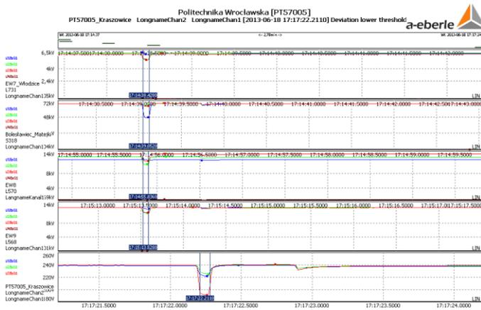
Figure 2. Synchronous registrations of a selected power quality disturbance seen at the measuring points of the system - a summary with time adjustment.
