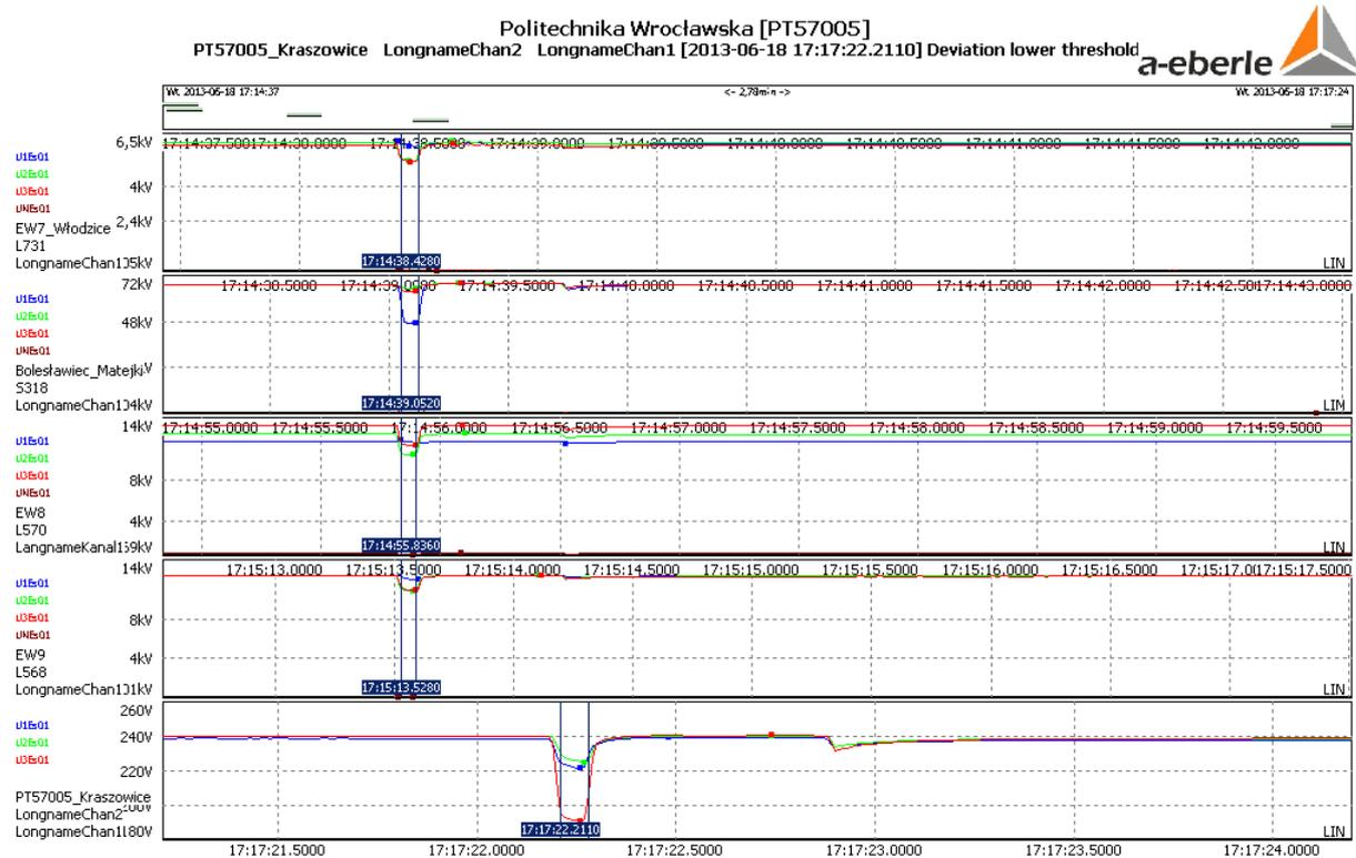
Figure 6. Synchronous registrations of a selected power quality disturbance seen at the measuring points of the system - a summary with time adjustment.
