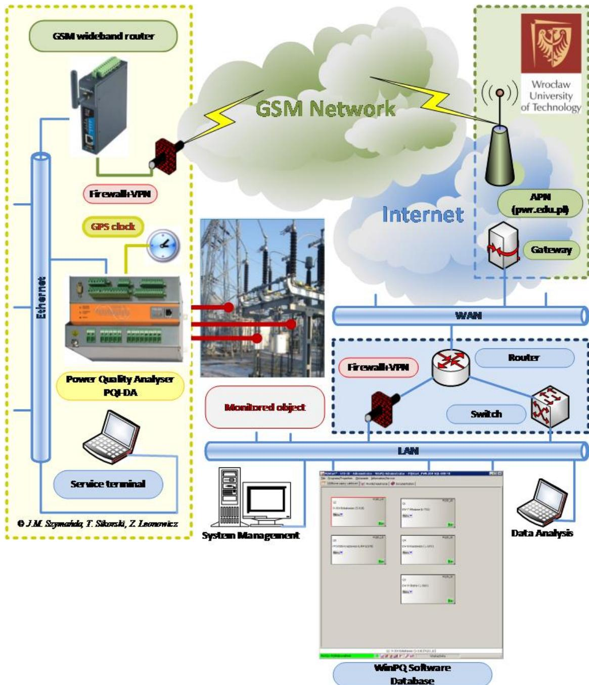
Figure 1. Functional diagram of the system.
