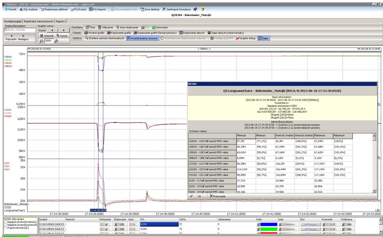
Figure 5. Registration of RecB RMS power quality disturbance recorded in the test point HV 110kV, Q2 and detailed parameters.
