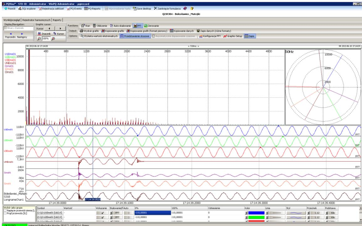
Figure 4. The selected recording of virtual oscilloscope RecA of power quality disturbances recorded in the test point HV 110kV, Q2, FFT frequency analysis and distribution of phasors.
