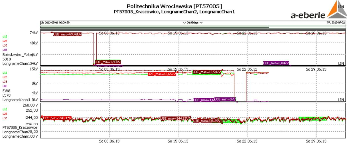
Figure 7. Data analysis tool with simultaneous creation of charts of selected parameters for many points on the example of aggregated 10-minute phase voltage measurement registered in points Q2, Q4 and Q5
