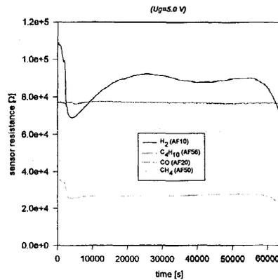
Fig. 3. Long-term sensor stability (standard heater supply voltage)
