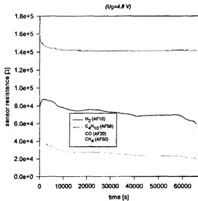
Fig. 2. Long-term sensor stability (low heater supply voltage)
