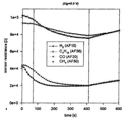
Fig. 5. Resistance responses - thermal extraction method
