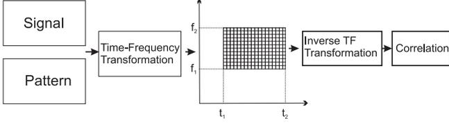
**Figure 1.** Scheme of correlation-based classification based on TF transformation.
